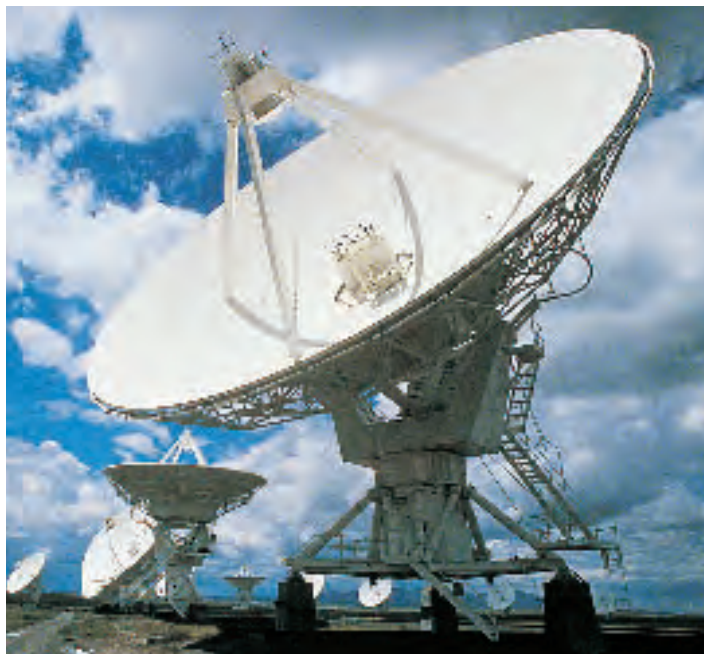
Figure 5 This radio telescope is used to study radio waves traveling through space.
