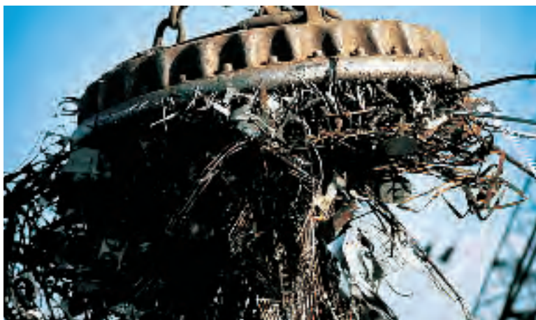
Figure 8 This junkyard magnet pulls scrap metal that can be salvaged from the rest of the debris. It is sorting by a physical property.
