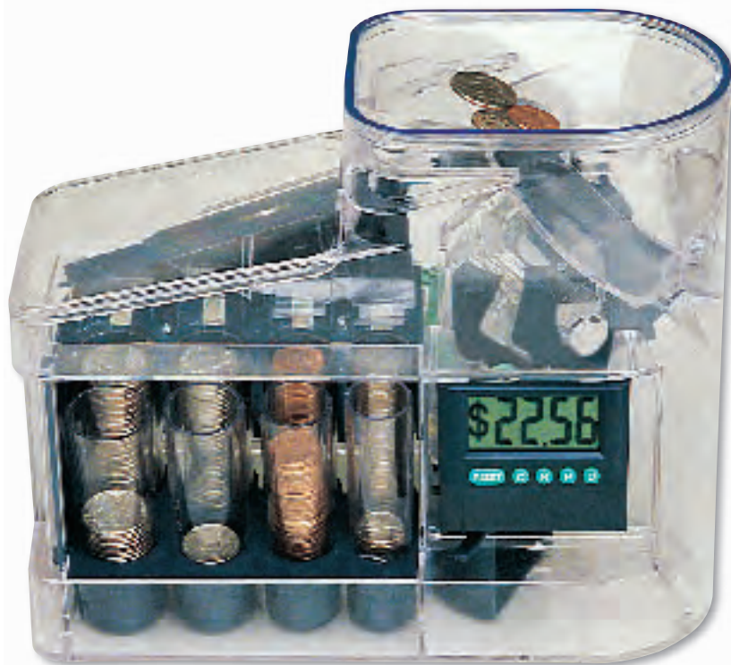
Figure 9 Coins can be sorted by their physical properties. Sorting by size is used here. Identify three other properties that can be used to sort coins.
