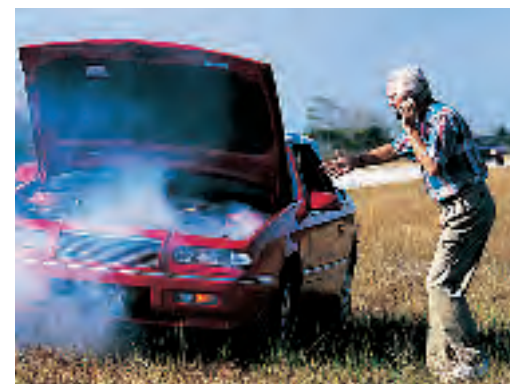
Figure 15 This car's engine overheated because its cooling system didn't carry enough heat from the engine.
