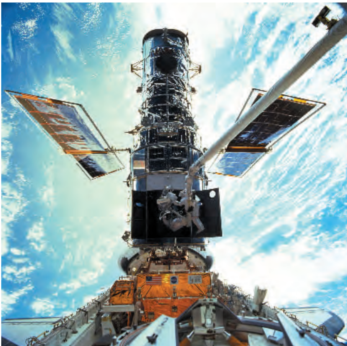
Figure 3 The Hubble Space Telescope was serviced at the end of 1999. Astronauts replaced devices on Hubble that are used to stabilize the telescope.
