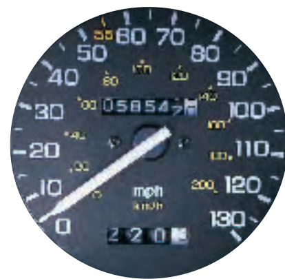
Figure 2 The odometer in a car measures the distance traveled. The speedometer measures instantaneous speed. Describe how you could use an odometer to measure average speed.
