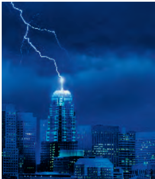
Figure 9 A lightning rod provides a path to conduct the charge in a lightning strike into the ground.
