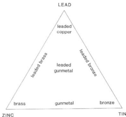
Figure 22. The different copper-based alloys as defined by Baley [102] for Roman Britain metalwork.
