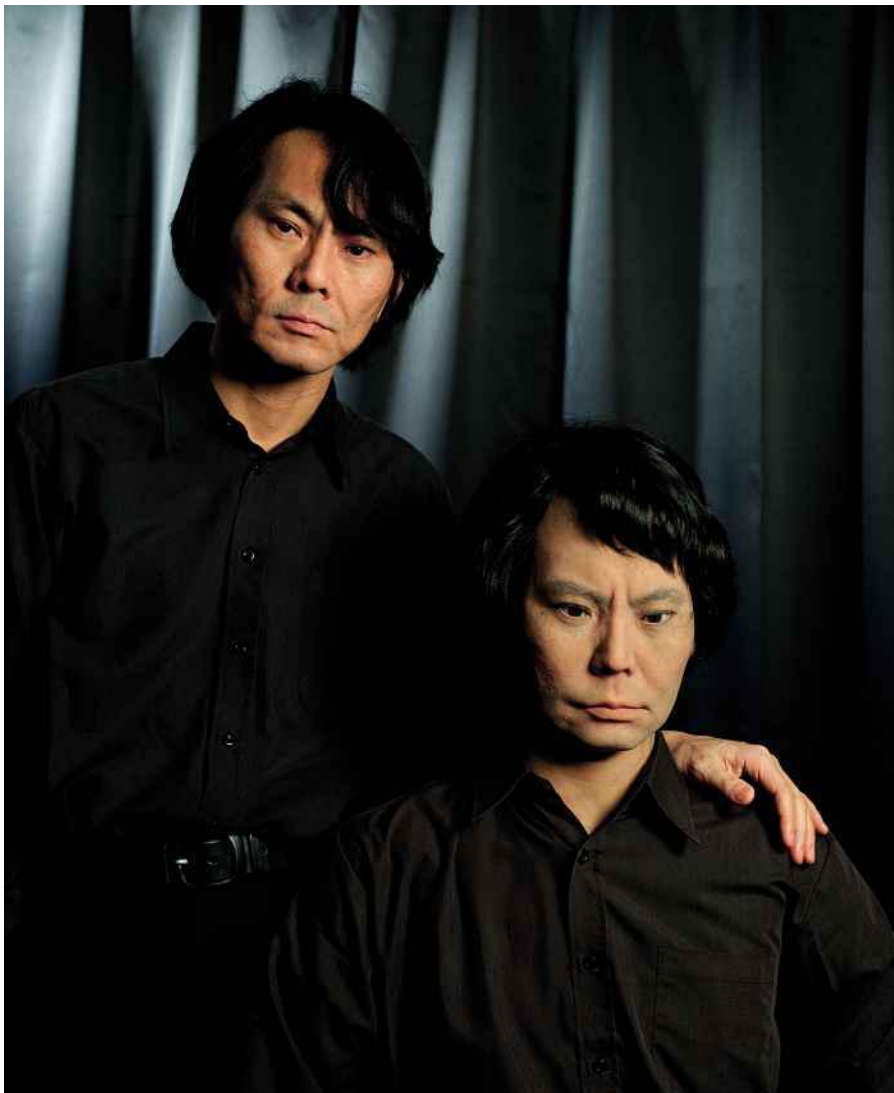
ABOVE: Professor Hiroshi Ishiguro poses with the Geminoid HI-4, an exact and remote-controlled replica of himself to test human-robot interaction and explore the uncanny valley.
