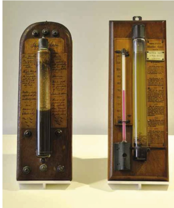
ABOVE: Two storm glasses, the one on the right designed by Admiral Robert Fitzroy.
