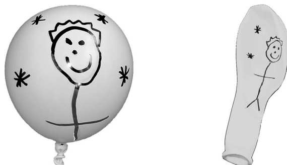
Figure 9.1 Changing materials by stretching
