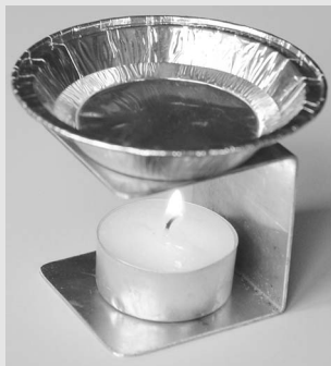
Figure 9.3 Evaporating a solution of salt and water
