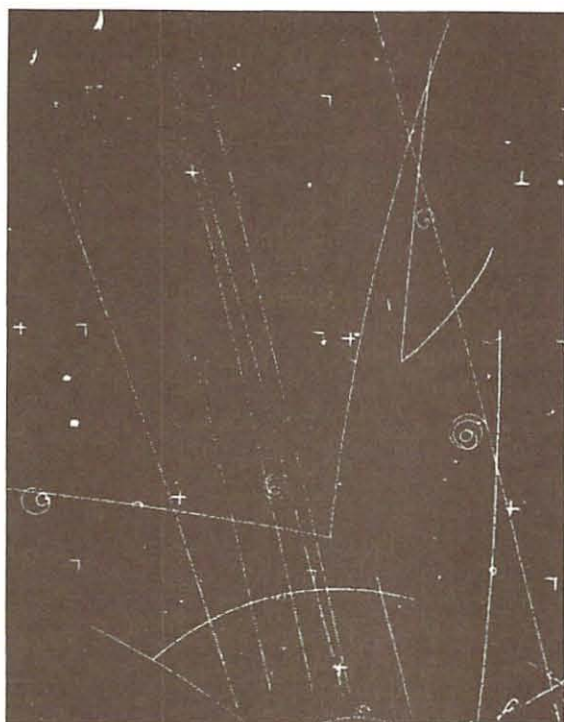
Figure 10.14 A hydrogen bubble chamber picture showing the reaction \pi^- + p \rightarrow \Lambda^0 + K^0 . Unlike the \pi^- and p , the \Lambda^0 and K^0 are neutral and do not leave a track of ions where bubbles start to form. The macroscopic distance between the formation and the decay of the \Lambda^0 and K^0 is indicative of the long lifetime of these hadrons. Image courtesy Lawrence Berkeley National Laboratory.
