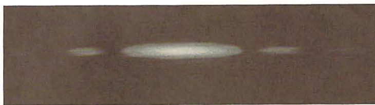
Figure 1.8 Diffraction pattern of laser light from a single slit. (Courtesy J. Newman)
