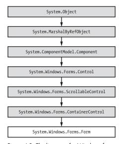
Figure 6-3: The lineage of a Windows form
