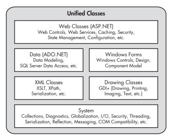
Figure 1-3: The unified classes in .NET
