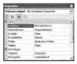
Figure 14-20: Making a file operation conditional
