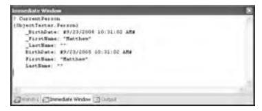
Figure 8-13: Printing an object's contents
