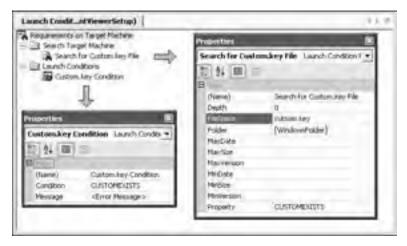
Figure 14-22: Anatomy of a launch condition that searches for a file
