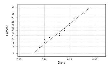
b) 95% two-sided confidence interval on mean rod diameter For  $\alpha=0.05$  and n=15,  $t_{\alpha/2,n-1}=t_{0.025,14}=2.145$
