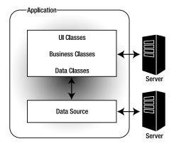
Figure 6-3. Two-tier design structure
