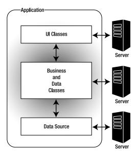
Figure 6-4. Three-tier design structure
