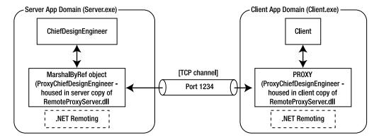
Figure 11-2. Remote-Proxy architecture
