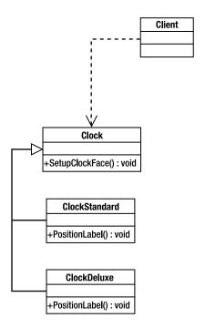
Figure 12-4. Template Method pattern
