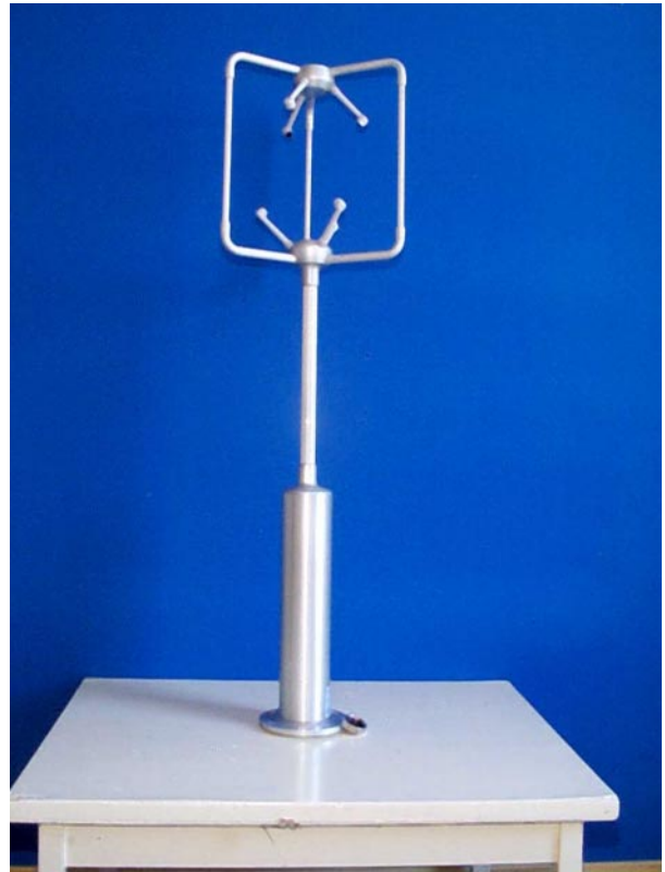
Figure 4 A commercially available pulse-type sonic anemometer. The three sets of paired transducers are capable of measuring the three components of the velocity vector. This type of device produced the time-series in Figure 1 and Figure 2 . The sonic anemometer measures 0.75 m from top to bottom.
