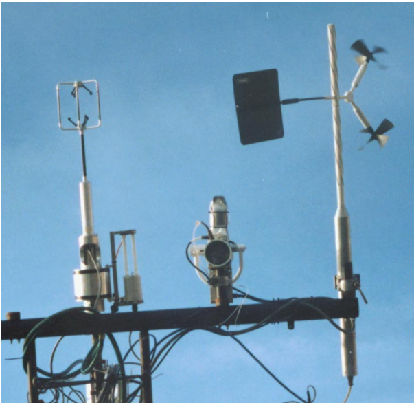
Figure 3 The instrument at the far right is a K-Gill anemometer shown during a deployment on a research vessel. The instrument on the left is a sonic anemometer that is shown in more detail in Figure 4 . Photograph provided by Olc Persson (CIRES/NOAA/ETL).
