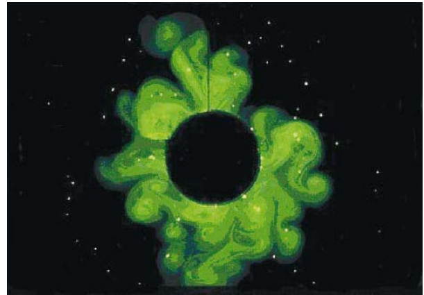
Figure 8 Eddies formed by cooling a rotating fluid in the laboratory. The dark central disk sits at the water surface and cools it, mimicking a region of cooling to the atmosphere. Coriolis forces give the thermal convection form, initially as small plumes (a few hundred meters across in the ocean), subsequently as mesoscale eddies with scale of 10–100 km, which dominate the scale model experiment here (oceanic flows and waves can be studied using scale models in the laboratory (e.g., Geophysical Fluid Dynamics Laboratory, University of Washington, http://www.ocean.washington.edu/research/gfd/gfd.html ).
