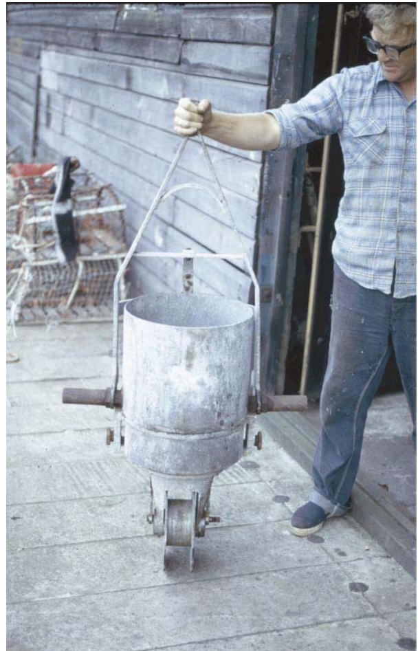
Figure 14 Knudsen sampler in ascent position.
