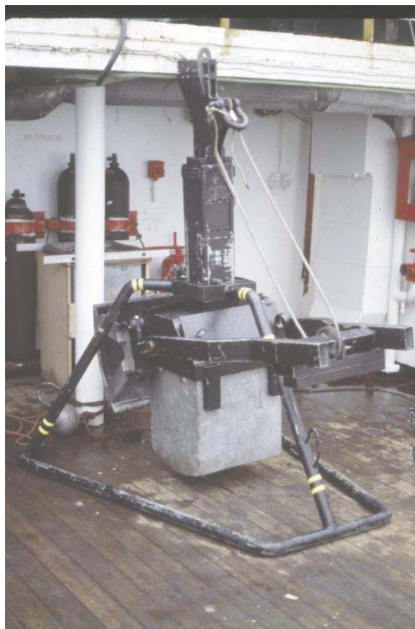
Figure 16 A 0.25\text{ m}^2 spade box sampler.
