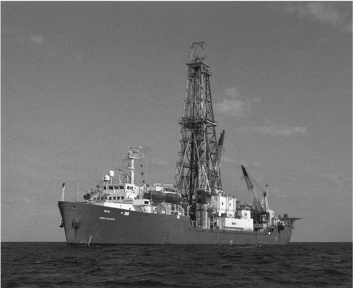
Figure 3 Scientific Research Vessel JOIDES Resolution operated by Transocean SedcoForex for the Ocean Drilling Program 1984 to present.
