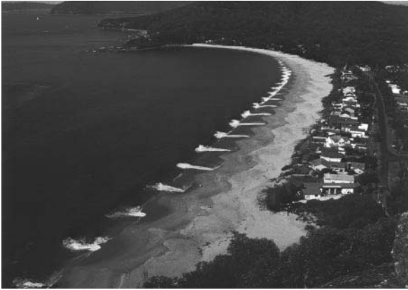
Figure 4 Pearl Beach near Sydney, Australia, is a modally reflective beach composed of medium to coarse sand and receiving usually lower swell waves. Note the very narrow zone of wave breaking, well-developed beach cusps and cusp-controlled segregated swash circulation (A.D. Short).
