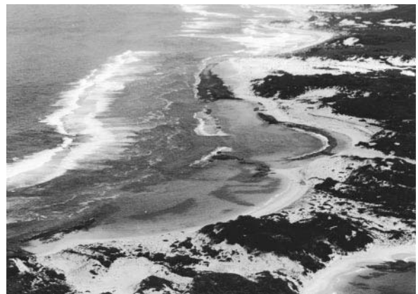
Figure 15 Three bands of beachrock at Shoal Cape, Western Australia. Note the wave breaking over the successive reefs, leading to a low energy inner beach, on an exposed high-energy coast (A.D. Short).
