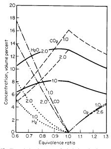
$\textbf{Fig. 9.6.15} \quad \text{Theoretical mole percent of principal combustion products of hydrocarbon fuels for fuel hydrogen/carbon ratios.}$
