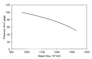
Fig. 9.1.18 Typical deliverability curve; steam flow to power plant [1,000 lb/h = (453 kg/h)] vs. turbine inlet pressure  $[100 \text{ lb/in}^2 \text{ gage } (689 \text{ kPa gage})]$ .
