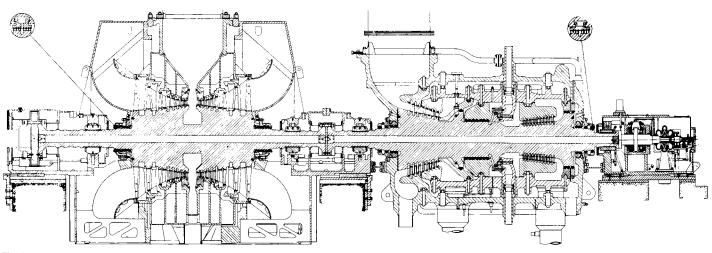
Fig. 9.4.11 Cross section of a 160,000-kW tandem-compound, double-flow reheat turbine. (Westinghouse Electric Corp.)
