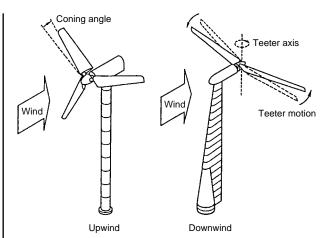
Fig. 9.1.6 HAWT configurations. (Courtesy of Atlantic Orient Corp.)
