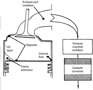
Fig. 9.6.63 Emission sources of unburned hydrocarbon and other organic gases. (Amann, "The Automotive Spark-Ignition Engine—An Historical Perspective," ASME-ICE vol. 8, 1989, pp. 33–45.)
