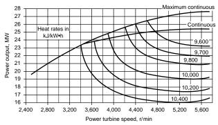
Fig. 9.7.23 Typical partial-load performance characteristics for variable output speed in a free-turbine drive.
