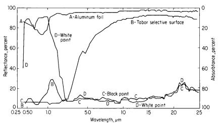
Fig. 9.1.12 Variation with wavelength of reflectance and absorptance for opaque surfaces.
