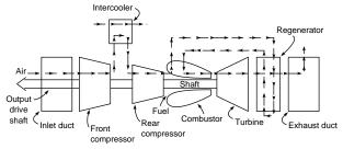
Fig. 9.7.13 Intercooled regenerative Brayton cycle gas-turbine component arrangement.
