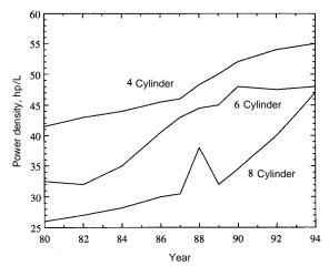
Fig. 9.6.17 Trend of average U.S. automobile power density.
