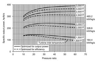
**Fig. 9.7.11** Intercooled Brayton cycle variation of specific output power with pressure ratio at different turbine inlet temperatures, optimized for output power and for efficiency.
