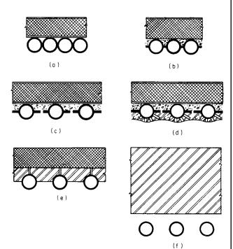
Fig. 9.2.27 Water-cooled furnace wall construction types. (a) Tangent tube wall; (b) welded membrane tube wall; (c) flat studs welded to sides of tubes; (d) full stud tube wall, refractory-covered; (e) tube and tile wall; (f) tubes spaced from refractory wall.
