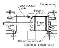
Fig. 9.3.3 Condensing uniflow engine cylinder, with clearance pockets.
