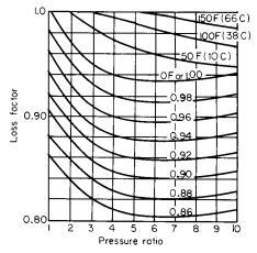
Fig. 9.4.7 Supersaturation and moisture loss.
