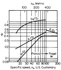
Fig. 9.9.7 Turbine characteristics and specific speed.
