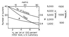
Fig. 9.9.13 Impulse turbine characteristics and proportions.
