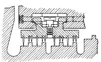
Fig. 9.4.14 Labyrinths with radial clearance.
