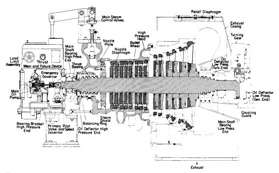
$\textbf{Fig. 9.4.10} \quad \text{Cross section of a multistage impulse condensing turbine rated at 30,000 kW.} \ \textit{(General Electric Co.)}$
