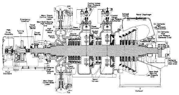
$\textbf{Fig. 9.4.16} \quad \text{Double automatic condensing extracting turbine, 25,000 kW.} \ \textit{(General Electric Co.)}$
