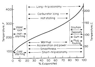
Fig. 9.6.30 Effects of volatility characteristics on engine performance.
