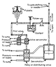
Fig. 9.9.19 Schematic diagram of governor.
