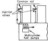
Fig. 9.6.43 Pump injection.
