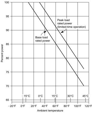
Fig. 9.7.24 Typical variation of output power with ambient temperature
