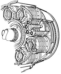
Can annular combustion chamber
