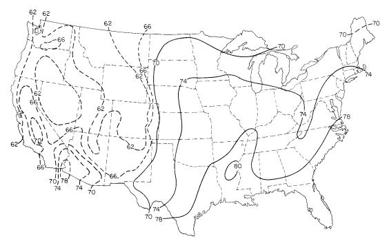
Fig. 9.5.21 Wet-bulb temperature, °F, isoclines at the 5 percent level, United States. (Adapted from Fluor Products Co., by permission.)
