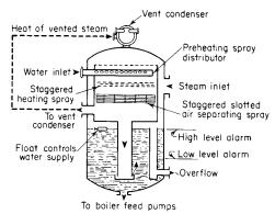
Fig. 9.5.33 Tray-type deaerating heater section.
