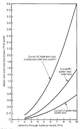
Fig. 9.5.11 Water-box and tube end losses, two-pass condensers. (Heat Exchange Institute.)
