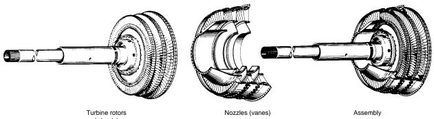
(wheels) Fig. 9.7.27 Turbine elements and assembly.
