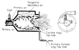
Fig. 9.2.16 Cyclone furnace.
