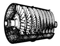
Fig. 9.7.25 Components and assembly of axial flow compressor.
