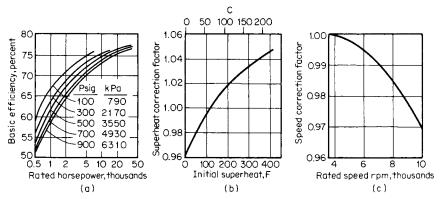
**Fig. 9.4.24** Mechanical-drive turbine efficiencies. (a) Basic efficiency, 3,600 r/min. Figures on curve are inlet steam pressure in lb/in² gage. (b) Superheat correction factor. (c) Rated-load speed-correction factor.
