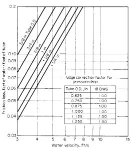
Fig. 9.5.7 Friction loss for water flowing in 18 BWG tubes, low velocity. (Heat Exchange Institute.)
