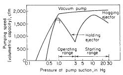
Fig. 9.5.18 Relative capabilities of air-removal pumps.
