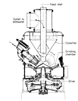
Fig. 9.2.11 Medium-speed pulverizer, roller type.
