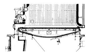
Fig. 9.2.8 Spreader stoker with traveling grate.
