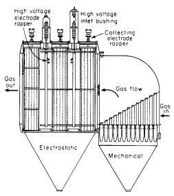
Fig. 9.2.7 Mechanical and electrostatic dust collectors in series.
