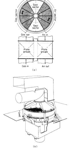
Fig. 9.2.32 Two designs of rotary regenerative air heaters.
