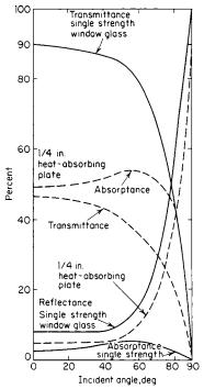
Fig. 9.1.11 Variation with incident angle of solar optical properties of  $3_{2}$ -in (2.4-mm) clear glass and 4-in (6.3-mm) heat-absorbing glass.
