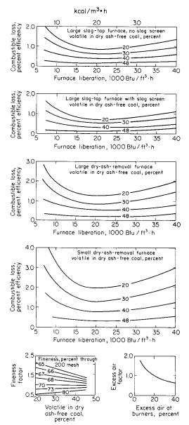
Fig. 9.2.17 Principal factors affecting combustible loss for pulverized coal firing in various types of furnaces.
