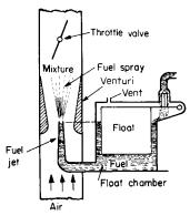
Fig. 9.6.38 Principle of carburetion.
