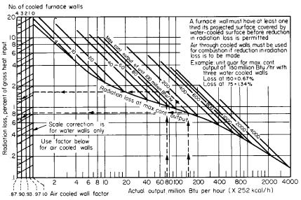
Fig. 9.2.37 External heat loss from boiler setting (ABMA).
