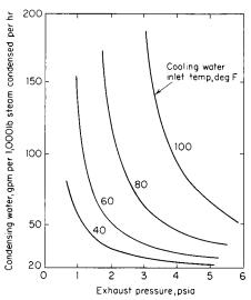
Fig. 9.5.14 Representative performance curves for a direct-contact condenser.
