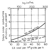
Fig. 9.2.18 Combustible efficiency loss, spreader stoker.
