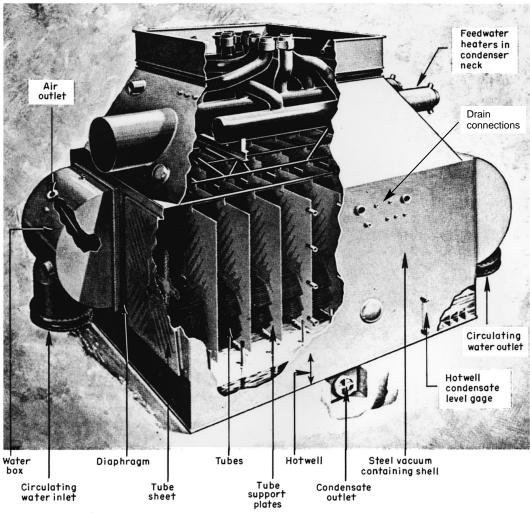
Fig. 9.5.2 One-pass rectangular surface condenser.
