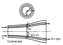
Fig. 9.1.3 Annular ring control volume.
