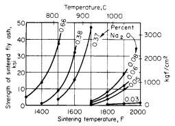
Fig. 9.2.3 Effect of sodium oxide content of coal on the sintered strength of fly
