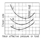
**Fig. 9.3.2** Engine steam rate curves (a) at the steam cylinder,  $lb/(ihp \cdot h)$ ; (b) at the engine shaft,  $lb/(bhp \cdot h)$ ; (c) at the generator, lb/kWh.
