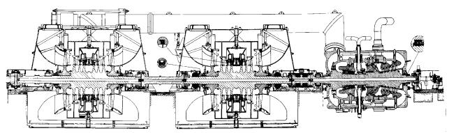
Fig. 9.4.18 Cross section of a 500-MW tandem-compound, quadruple-flow 3,600-r/min reheat turbine. (Westinghouse Electric Corp.)
