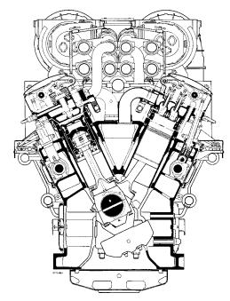
Fig. 9.6.23 Cross section of Sulzer V-type ZV-40 engine. Bore = 400 mm; stroke = 480 mm.
