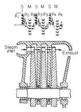
Fig. 9.4.1 Impulse turbine with single-velocity stages.
