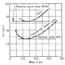
Fig. 9.3.8 Theoretical and test steam rate curves. Uniflow engine  $20 \times 24$  at 200 r/min; throttle conditions 150 lb/in<sup>2</sup> saturated steam; exhaust to atmosphere.
