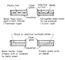
Fig. 9.1.14 Typical flat-plate solar radiation collectors.
