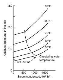
Fig. 9.5.5 Representative performance curves for a 157,500-ft<sup>2</sup> one-pass surface condenser, 1-in, 18-gage, 37.8-ft-active-length aluminum-brass tubes. Performance is based on 85 percent clean tubes, 221,400 gal/min cooling water at a velocity of 7 ft/s, and 968 Btu/lb rejected to the cooling water.
