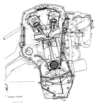
Fig. 9.6.18 Oldsmobile Division Quad 4 with four valves per cylinder (1987).
