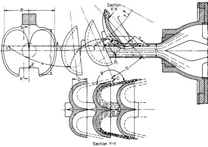
Fig. 9.9.14 Impulse turbine bucket design.
