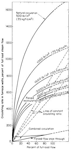
Fig. 9.2.36 Circulating flow for natural- and forced-circulation systems.
