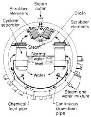
$\label{eq:Fig. 9.2.38} \textbf{ Prum internal arrangement with cyclone steam separators and scrubber elements.}$
