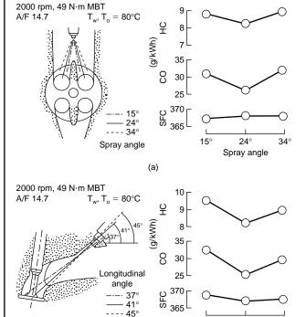
Fig. 9.6.42 Effects of spray angle and injection targeting on engine emissions. (a) Effect of dual stream separation angle; (b) effect of injection direction. (Iwata et al., SAE paper 870125, 1987.)
