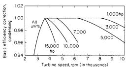
Fig. 9.4.23 Correction factor for condensing mechanical-drive turbines.
