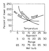
Fig. 9.5.24 Comparative cooling tower costs. (Foster Wheeler Corp.)
