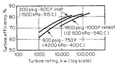
Fig. 9.4.22 Turbine efficiencies vs. capacity.
