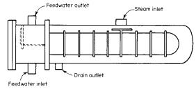
Fig. 9.5.26 Basic heater section for condensing heater.
