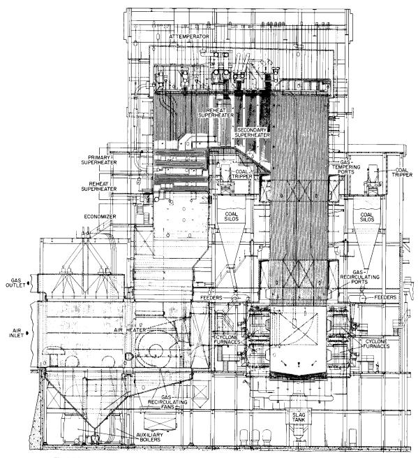
$\label{eq:fig.9.2.24} Universal Pressure boiler; pressurized cyclone furnace, coal-fired; 8,000,000 lb (3,640 t) steam per hour; 3,650 lb/in² (257 kgf/cm²) pressure; 1,003°F (539°C) steam temperature; 1,003°F (539°C) reheat steam temperature.$
