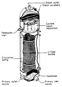
Fig. 9.2.40 Nuclear power boiler.
