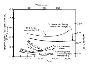
Fig. 9.6.26 Specific fuel consumption curves.
