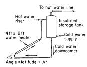
Fig. 9.1.16 Thermosiphon type of water heater. (\*The collector angle A depends on the latitude. More favorable orientation toward the winter sun when days are shorter can produce the same amount of hot water all year round. In Florida, A is  $10^{\circ}$ .)
