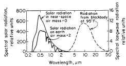
Fig. 9.1.10 Spectral distribution of solar radiation and radiation emitted by blackbody at  $95^{\circ}F$  ( $35^{\circ}C$ ).
