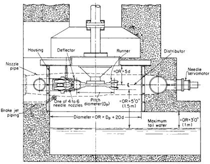
Fig. 9.9.12 Vertical-shaft multijet impulse turbine installation.
