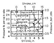
Fig. 9.6.12 Pumping loop of Otto cycle engine.
