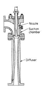
Fig. 9.5.17 Single-stage air ejector.
