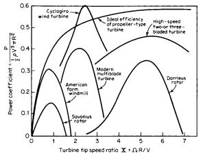
Fig. 9.1.2 Performance curves for wind turbines.
