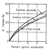
Fig. 9.6.61 Improvement in CN with ignition accelerators. (Bogen and Wilson.)
