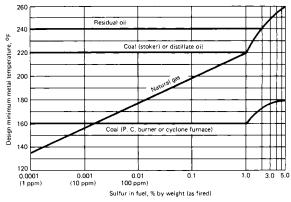
Fig. 9.2.30 Limiting metal temperatures to avoid external corrosion in economizers or air heaters when fuel containing sulfur is burned.
