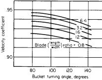
Fig. 9.4.5 Impulse-bucket velocity coefficients.
