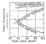
Fig. 9.2.29 Comparative radiant and convection superheater characteristics.
