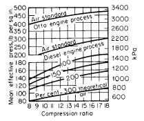
Fig. 9.6.9 MEP for diesel cycle engine [air and liquid dodecane supplied at  $60^{\circ}F$  ( $16^{\circ}C$ )].
