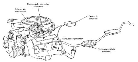
Fig. 9.6.66 Closed-loop three-way catalyst (TWC) system.
