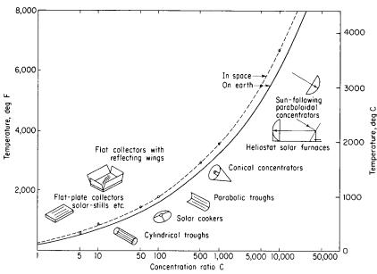
Fig. 9.1.13 Variation with concentration ratio of equilibrium temperatures for earth and space.
