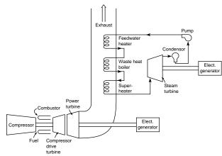
Fig. 9.7.18 Schematic of combined-cycle heat recovery system.
