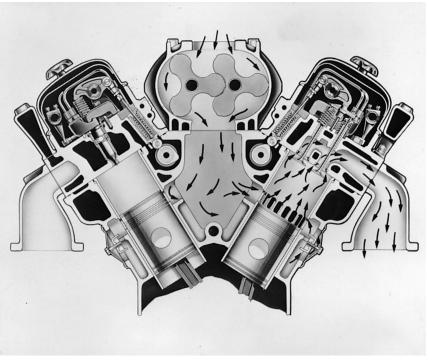
Fig. 9.6.20 Blower-scavenged Detroit diesel model 8V-71N two-stroke diesel engine.
