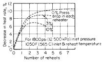
Fig. 9.4.25 Approximate gains due to reheating.
