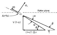
Fig. 9.1.4 Velocity and force vector diagrams.
