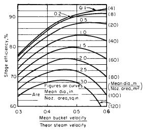
Fig. 9.4.6 Turbine single-row stage efficiency.
