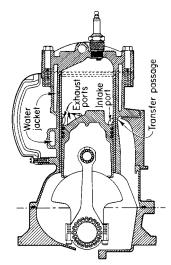
Fig. 9.6.24 Johnson two-cycle, 30-hp outboard motor.
