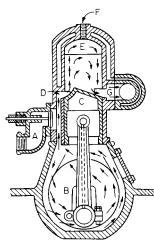
Fig. 9.6.5 Small two-cycle gasoline engine with crankcase compression.
