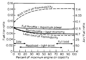
Fig. 9.6.37 Mixture ratios for spark ignition engines.
