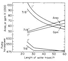
Fig. 9.5.12 Condenser configuration selection for a given heat load,  $W_s =$ 477,355 lb/h; h = 975 Btu/lb;  $t_i = 70.0$ °F; 1.5 inHg abs; 18-gage admiralty metal tubes; 7.0-ft/s water velocity; 85 percent cleanliness factor.
