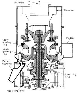
Fig. 9.2.10 Medium-speed pulverizer, contrarotation ball-and-race type.
