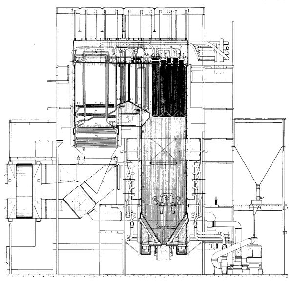
Fig. 9.2.23 Once-through boiler with combined circulation; twin pressurized furnaces; pulverized coal tangentially fired; 6,400,000 lb (2,900 t) steam per hour; 3,650 lb/in<sup>2</sup>  $(257 \text{ kgf/cm}^2)$  pressure;  $1,003^{\circ}\text{F}$   $(539^{\circ}\text{C})$  steam temperature;  $1,003^{\circ}\text{F}$   $(539^{\circ}\text{C})$  reheat steam temperature.
