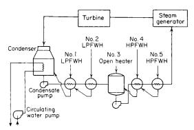
Fig. 9.5.1 Equipment arrangement, schematic.
