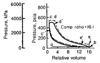
**Fig. 9.6.2** Diesel cycle (constant-pressure combustion, 50 percent excess air). Processes of the ideal cycle: *a-b*, suction stroke, admission of air; *b-c*, compression of air; *c-d*, injection and combustion of the fuel; *d-e*, expansion; at *e*, exhaust valve opens; *b-a*, exhaust stroke.
