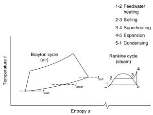
Fig. 9.7.19 Combined-cycle temperature vs. entropy diagram.
