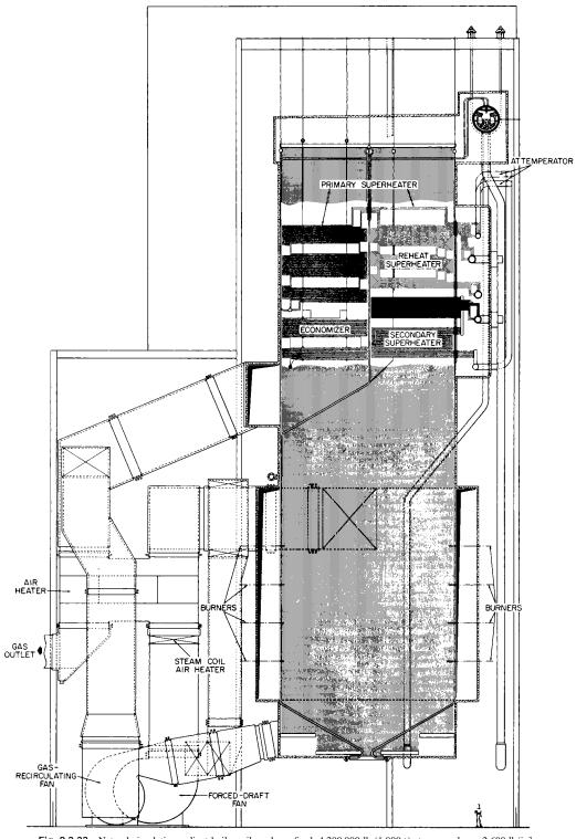
$\label{eq:fig.9.2.22} Natural circulation radiant boiler, oil- and gas-fired; 4,200,000 lb (1,900 t) steam per hour; 2,600 lb/in^2 (183 kgf/cm^2) pressure; 1,005°F (540°C) steam temperature; 1,005°F (540°C) reheat steam temperature.$
