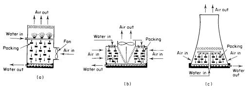
Fig. 9.5.22 Cooling tower types. (a) Forced draft; (b) crossflow-induced draft; (c) hyperbolic.
