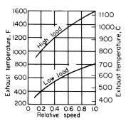
Fig. 9.6.13 Exhaust temperatures for Otto cycle engines.
