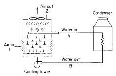
Fig. 9.5.19 Schematic for induced-draft, counterflow, cooling tower installa-
