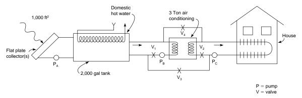
Fig. 9.1.17 Schematic of typical solar house heating, cooling, and hot water system.
