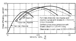
Fig. 9.4.9 Variation of the efficiency of turbine elements with velocity ratio.
