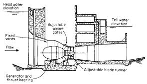
Fig. 9.9.4 Axial-flow bulb turbine.
