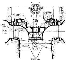
Fig. 9.9.3 Adjustable-blade Kaplan turbine.
