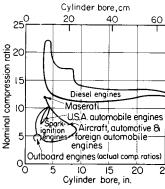
Fig. 9.6.62 Range of compression ratios as a function of cylinder bore.
