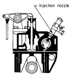
Fig. 9.6.54 Ricardo divided combustion chamber.
