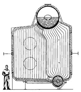
Fig. 9.2.20 Water-tube package boiler, single-pass gas.
