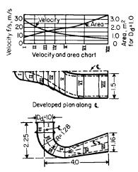
Fig. 9.9.11 Elbow draft tube layout.
