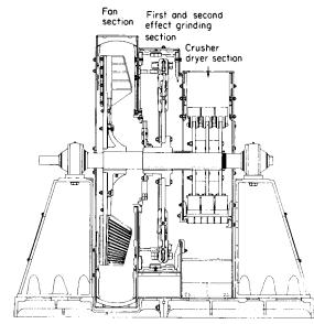
Fig. 9.2.12 High-speed pulverizer, attrition type.
