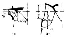
Fig. 9.9.2 Typical profile of Francis runners. (a) Low specific speed; (b) high specific speed.
