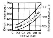
Fig. 9.6.14 Exhaust temperatures for diesel cycle engines.
