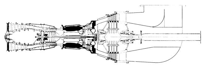
Fig. 9.7.1 Cross section of Pratt and Whitney FT8 gas turbine derived from the JT8D commercial aircraft engine.
