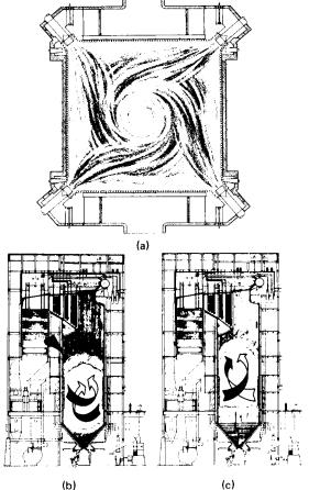
Fig. 9.2.15 Corner fired tangential tilting burners for pulverized coal, oil, or gas. (a) Plan section; (b) burners tilted down; (c) burners tilted up.
