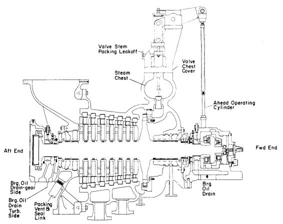
Fig. 9.4.17a A 16,000-hp cross-compound marine turbine designed for steam conditions of 600 lb/in<sup>2</sup> gage, 850°F,  $1\frac{1}{2}$  inHg abs. High-pressure section for 6,550-r/min normal speed. Low-pressure section in Fig. 9.4.17b. (General Electric Co.)
