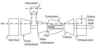
Fig. 9.7.9 Intercooled Brayton cycle gas-turbine component arrangement.
