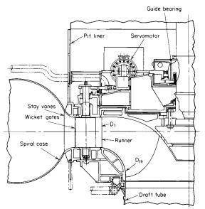
Fig. 9.9.15 Reversible pump turbine.
