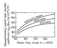
Fig. 9.5.31 Approximate desuperheater section heat-transfer rates.
