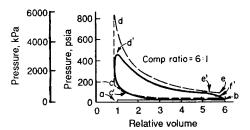
Fig. 9.6.1 Otto cycle (constant-volume combustion, no excess air). Process of the ideal cycle: a-b, suction stroke, admission of the charge; b-c, compression stroke; at c, ignition of the compressed charge; d-e, expansion; at e, exhaust valve opens; b-a, exhaust stroke.
