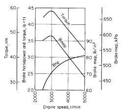
Fig. 9.6.25 Performance of Johnson outboard motor.
