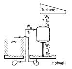
Fig. 9.5.15 Direct-contact condenser performance terms.
