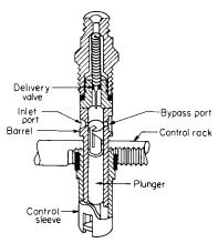
Fig. 9.6.45 Bosch plunger, barrel, and delivery valve assembly.
