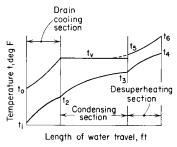
Fig. 9.5.28 Temperature vs. water travel, closed-feed heater.
