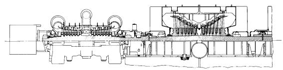
Fig. 9.4.19 Cross section of a 1,300-MW class tandem-compound, six-flow 1,800-r/min turbine for steam from light-water nuclear reactors, showing one of the three low-pressure sections. (General Electric Co.)
