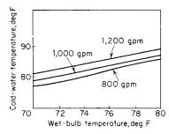
Fig. 9.5.23 Cooling tower performance. Design for  $85^{\circ}F$  cold water,  $95^{\circ}F$  hot water,  $78^{\circ}F$  wet-bulb temperature,  $10^{\circ}$  range; 1,000-gal/min cell.
