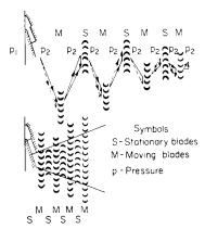
Fig. 9.4.2 Impulse turbine with multivelocity stages.
