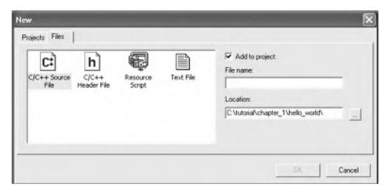
The defaults are correct (or they should be). You are creating a C/C++ source file and adding it to the project; the location of the file is the same place that you placed the project itself. All you need to do is give the file a name. Type hellomain into the File name box. After I have opened the FileView tree (in the left-hand pane), the top left of my work window looks like this:
