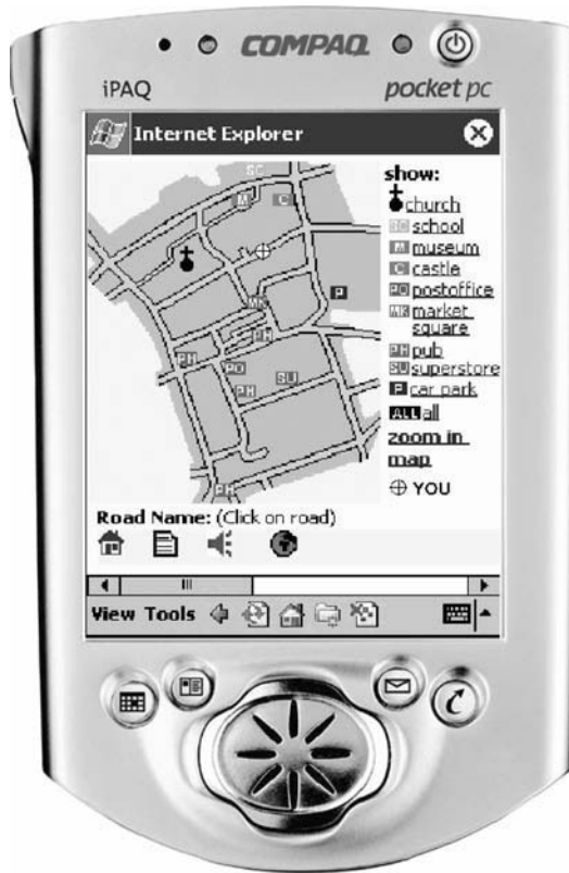
Fig. 32.2 Experimental PDA interface for LBS that provides map, text and voice wayfinding instructions
