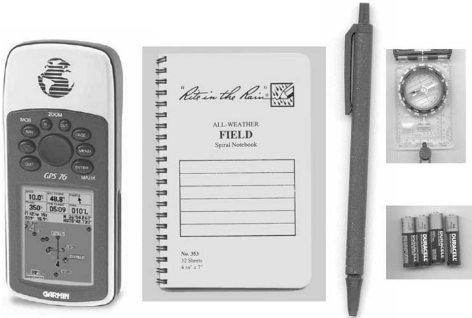
Fig. 28.7 Waterproof kit contents: GPS receiver, field notebook, pencils, compass, and extra batteries
