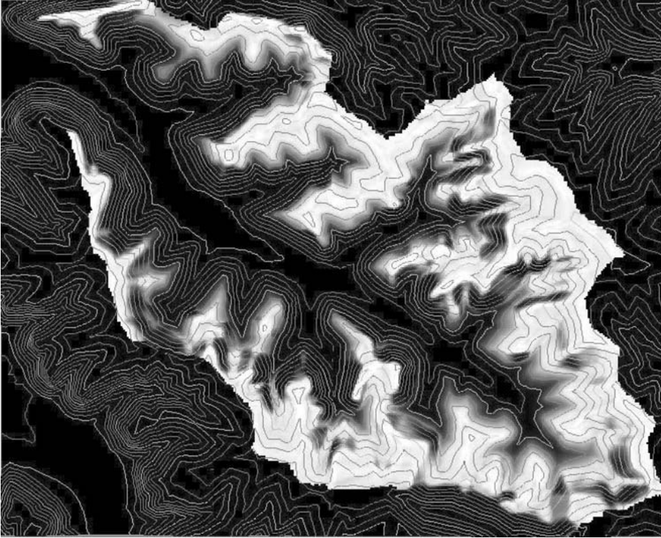
Fig. 15.6 The predicted distribution of Soil Series Basco in Pleasant Valley, Wisconsin, USA based on a fuzzy implementation of the rule in Figure 15.2. The lighter the grades the more typical of Basco (thin lines are contours)
