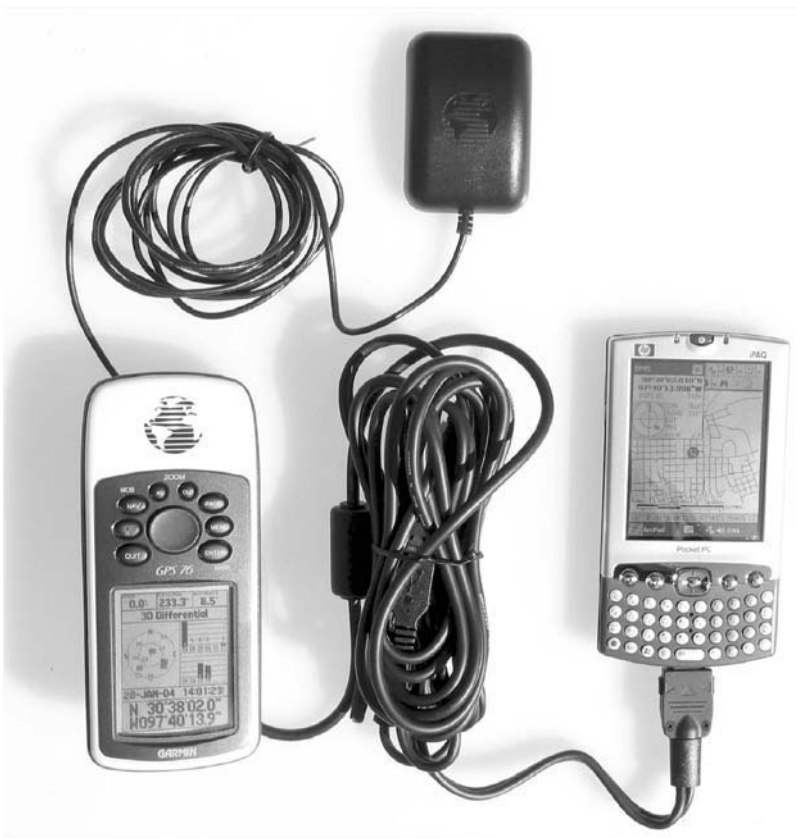
Fig. 28.8 DGPS receiver and pocket PC with ArcPad data collection software
