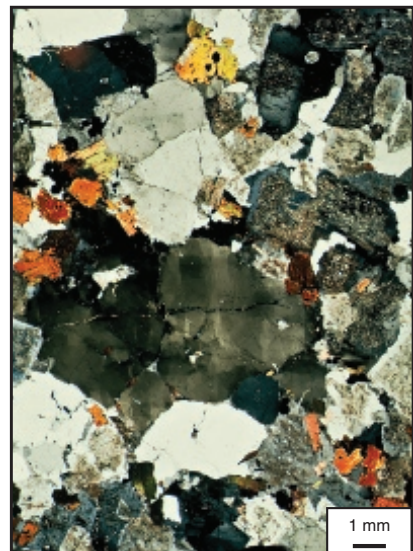
56 Quartz in a granite with polars crossed.
