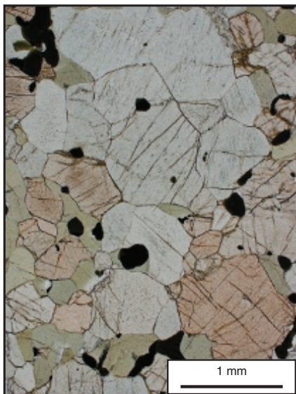
247 & 248 Orthopyroxene-clinopyroxene granofels in plane-polarized light and crossed-polars.
