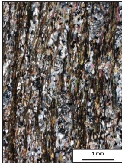
185 Mica schist in crossed polars showing a spaced schistosity.
