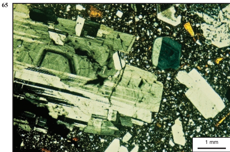
65 Zoned plagioclase phenocryst in a lava with crossed polars.
