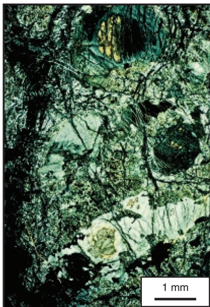
259 & 260 Lizardite Serpentinite in plane-polarized light and crossed-polars. Locality: Lizard Head, Cornwall, England.
