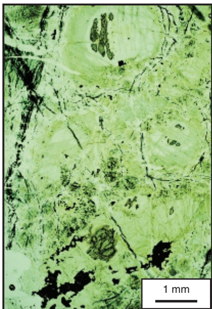
259 & 260 Lizardite Serpentinite in plane-polarized light and crossed-polars. Locality: Lizard Head, Cornwall, England.
