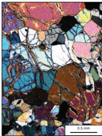
31 Olivine in a peridotite in crossed polars.
