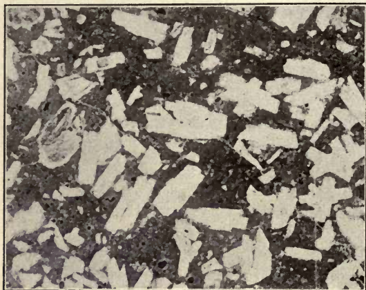
FIG. 369.—Porphyritic Feldspar Crystals in a Fine Grained Crystalline Ground Mass.
