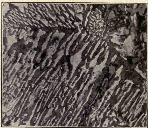
FIG. 370.—Section of a Micropegmatite enlarged, showing Eutectic Structure.
