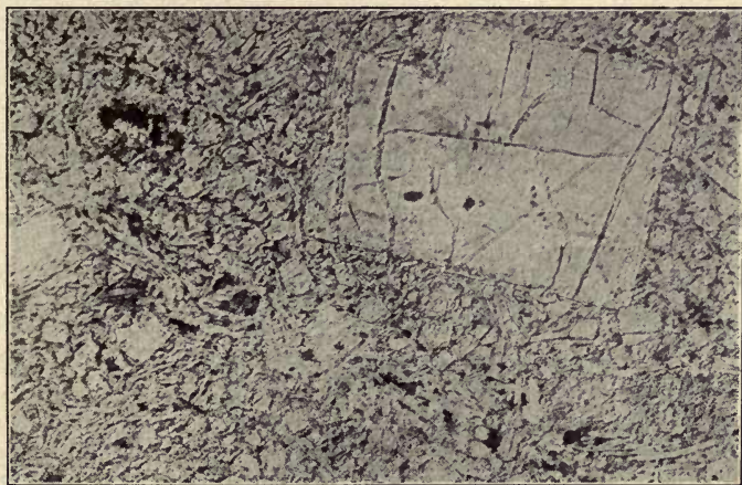
FIG. 482. — Nepheline in a Section of Phonolite. The Small Square Crystals are also Nepheline. The Elongated Crystals are Feldspar.
