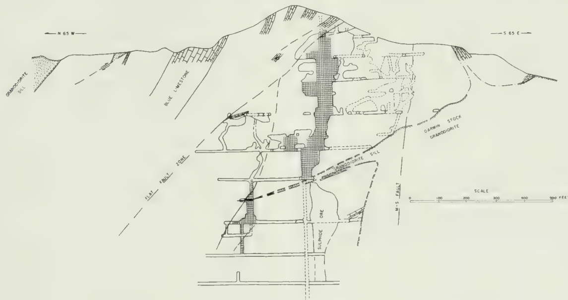
FIGURE 3. Longitudinal section of the Essex ore zone, Darwin mines. After Davis and Peterson, 1949.
