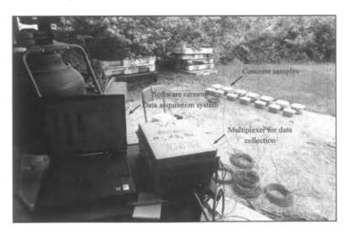
Figure 1 Curing of concrete specimens in outdoor environment
