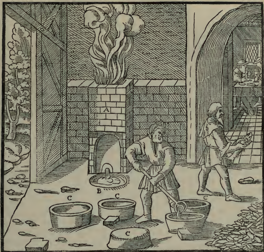
A—FURNACE. B—FOREHEARTH. C—OBLONG MOULDS.
