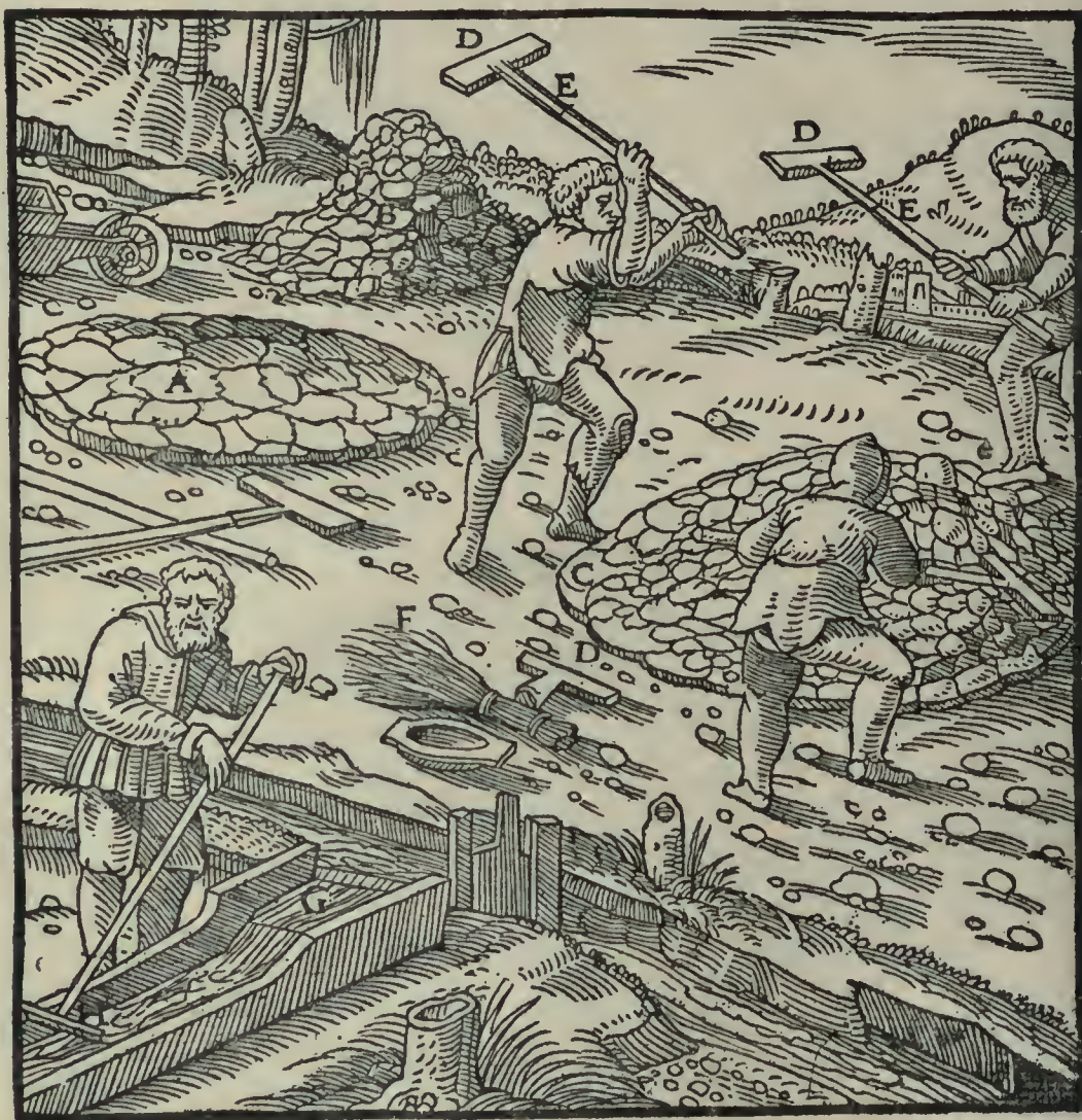
A—AREA PAVED WITH STONES. B—BROKEN ORE. C—AREA COVERED WITH BROKEN ORE. D—IRON TOOL. E—ITS HANDLE. F—BROOM. G—SHORT STRAKE. H—WOODEN HOE.
