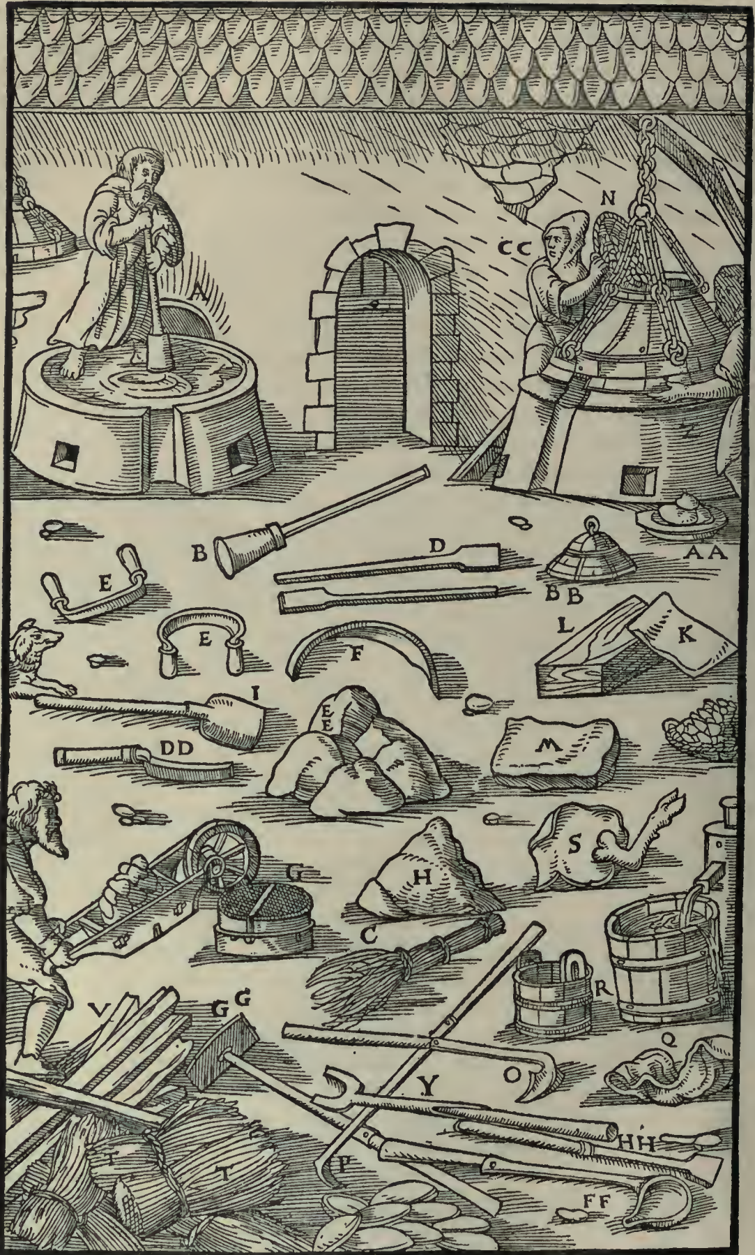
A—AN ARTIFICER TAMPING THE CRUCIBLE WITH A RAMMER. B—LARGE RAMMER. C—BROOM. D—TWO SMALLER RAMMERS. E—CURVED IRON PLATES. F—PART OF A WOODEN STRIP. G—SIEVE. H—ASHES. I—IRON SHOVEL. K—IRON PLATE. L—BLOCK OF WOOD. M—ROCK. N—BASKET MADE OF WOVEN TWIGS. O—HOOKED BAR. P—SECOND HOOKED BAR. Q—OLD LINEN RAG. R—BUCKET. S—DOESKIN. T—BUNDLES OF STRAW. V—WOOD. X—CAKES OF LEAD ALLOY. Y—FORK. Z—ANOTHER WORKMAN COVERS THE OUTSIDE OF THE FURNACE WITH LUTE WHERE THE DOME FITS ON IT. AA—BASKET FULL OF ASHES. BB—LID OF THE DOME. CC—THE ASSISTANT STANDING ON THE STEPS POURS CHARCOAL INTO THE CRUCIBLE THROUGH THE HOLE AT THE TOP OF THE DOME. DD—IRON IMPLEMENT WITH WHICH THE LUTE IS BEATEN. EE—LUTE. FF—LADLE WITH WHICH THE WORKMAN OR MASTER TAKES A SAMPLE. GG—RABBLE WITH WHICH THE SCUM OF IMPURE LEAD IS DRAWN OFF. HH—
