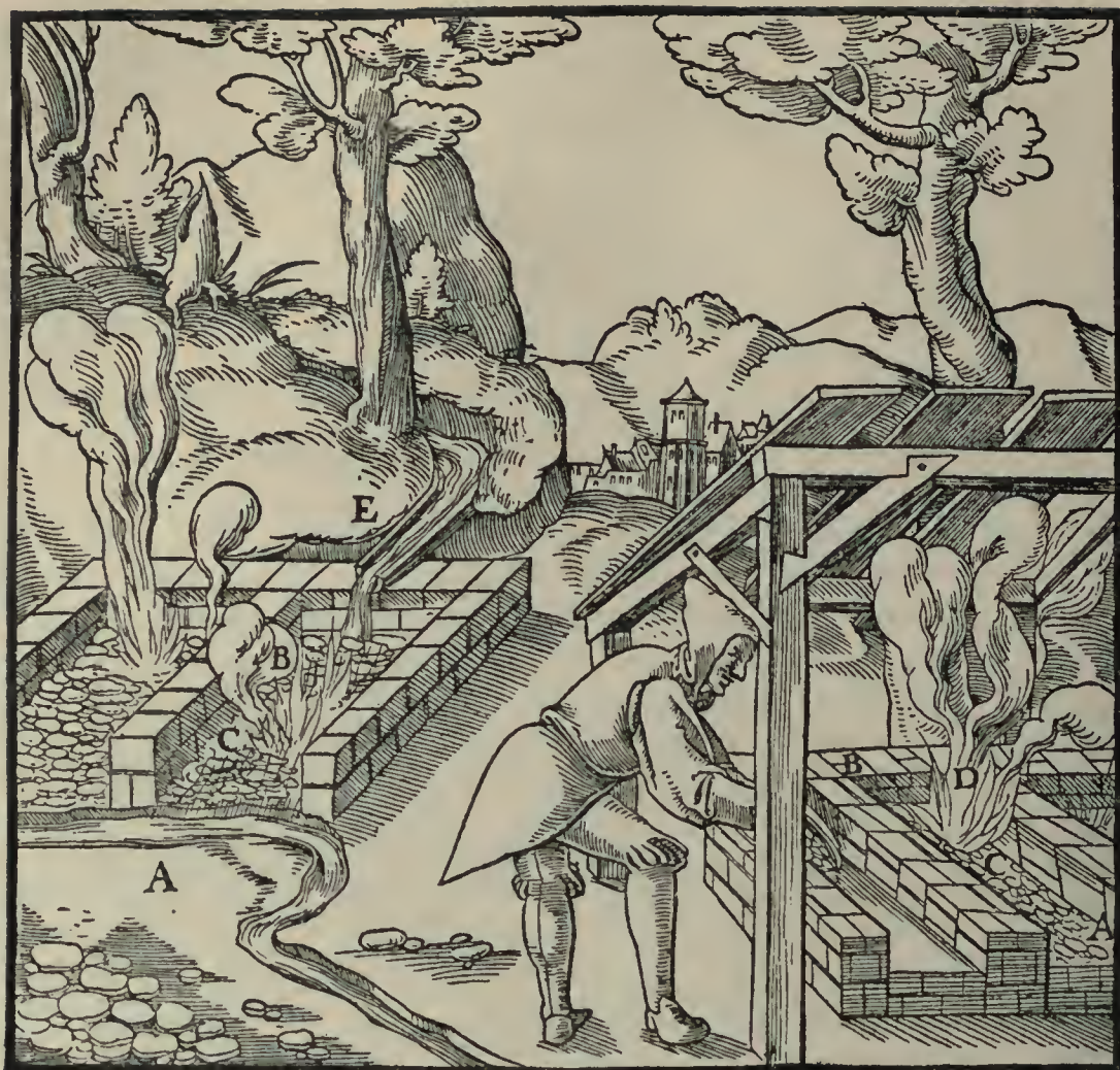
A—AREA. B—WOOD. C—ORE. D—CONE-SHAPED PILES. E—CANAL.
