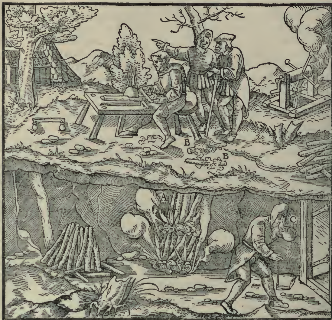
A—KINDLED LOGS. B—STICKS SHAVED DOWN FAN-SHAPED. C—TUNNEL.
