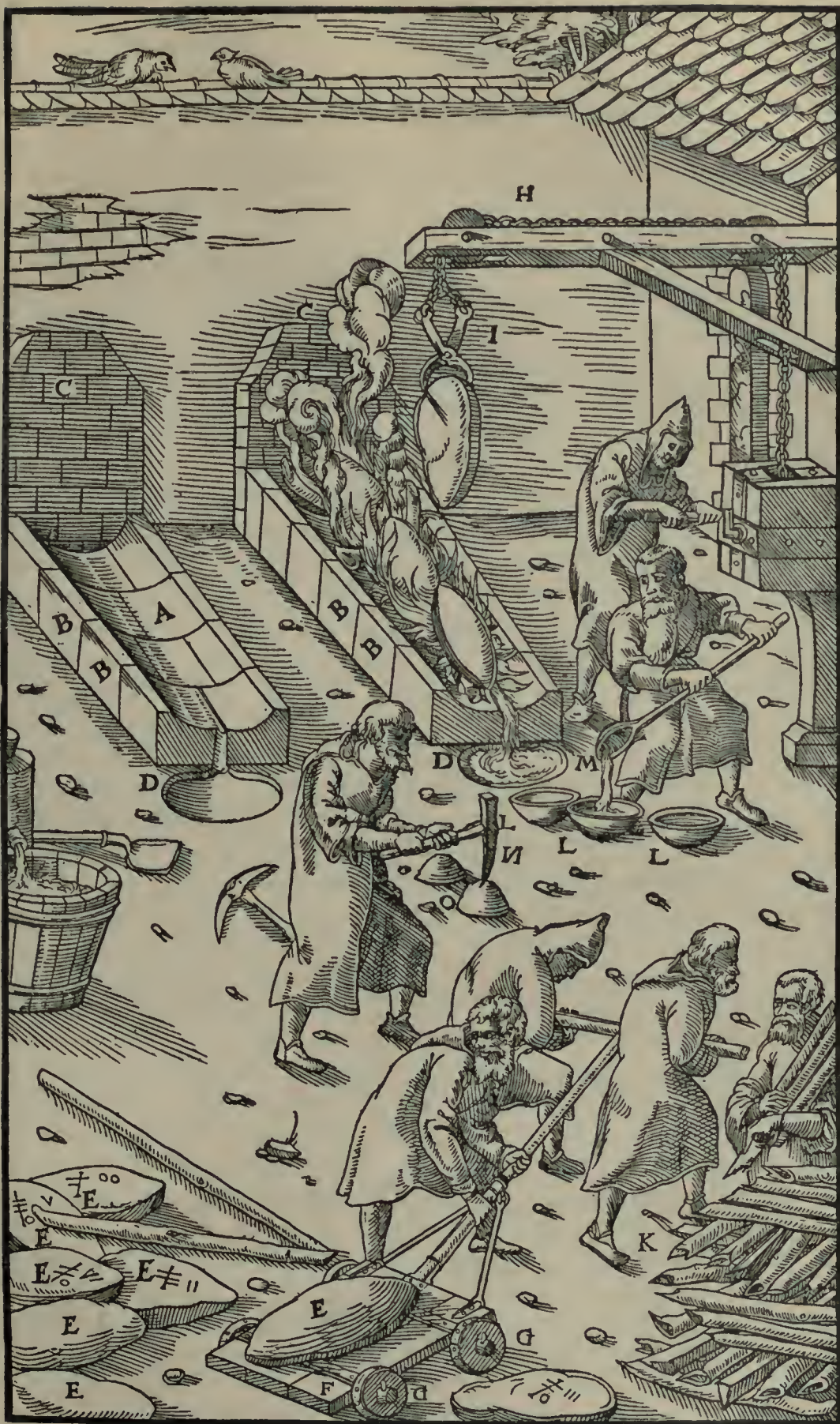
A—HEARTH. B—ROCKS SUNK INTO THE GROUND. C—WALLS WHICH PROTECT THE FOURTH LONG WALL FROM DAMAGE BY FIRE. D—DIPPING-POT. E—MASSES OF LEAD. F—TROLLEY. G—ITS WHEELS. H—CRANE. I—TONGS. K—WOOD. L—MOULDS. M—LADLE. N—PICK. O—CAKES.
