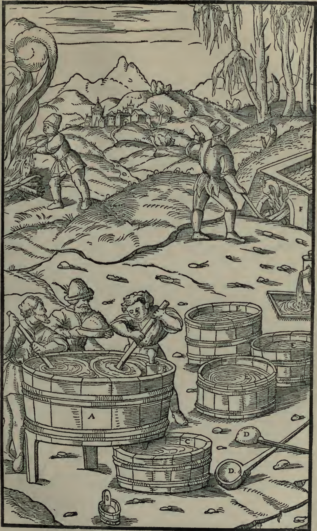
A—LARGE VAT. B—PLUG. C—SMALL TUB. D—DEEP LADLE. E—SMALL VAT. F—CALDRON.
