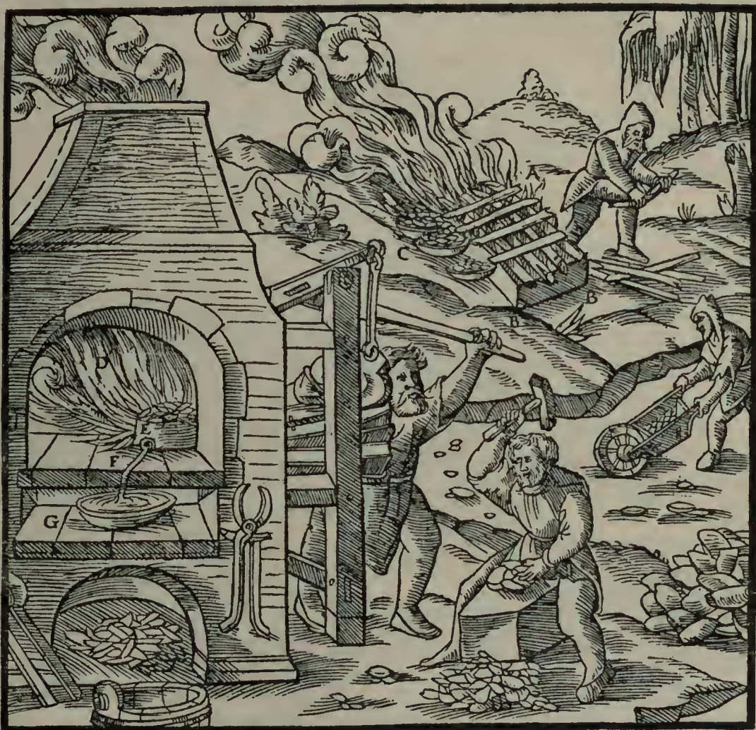
A—WOOD. B—BRICKS. C—PANS. D—FURNACE. E—CRUCIBLE. F—PIPE. G—DIPPING-POT.
