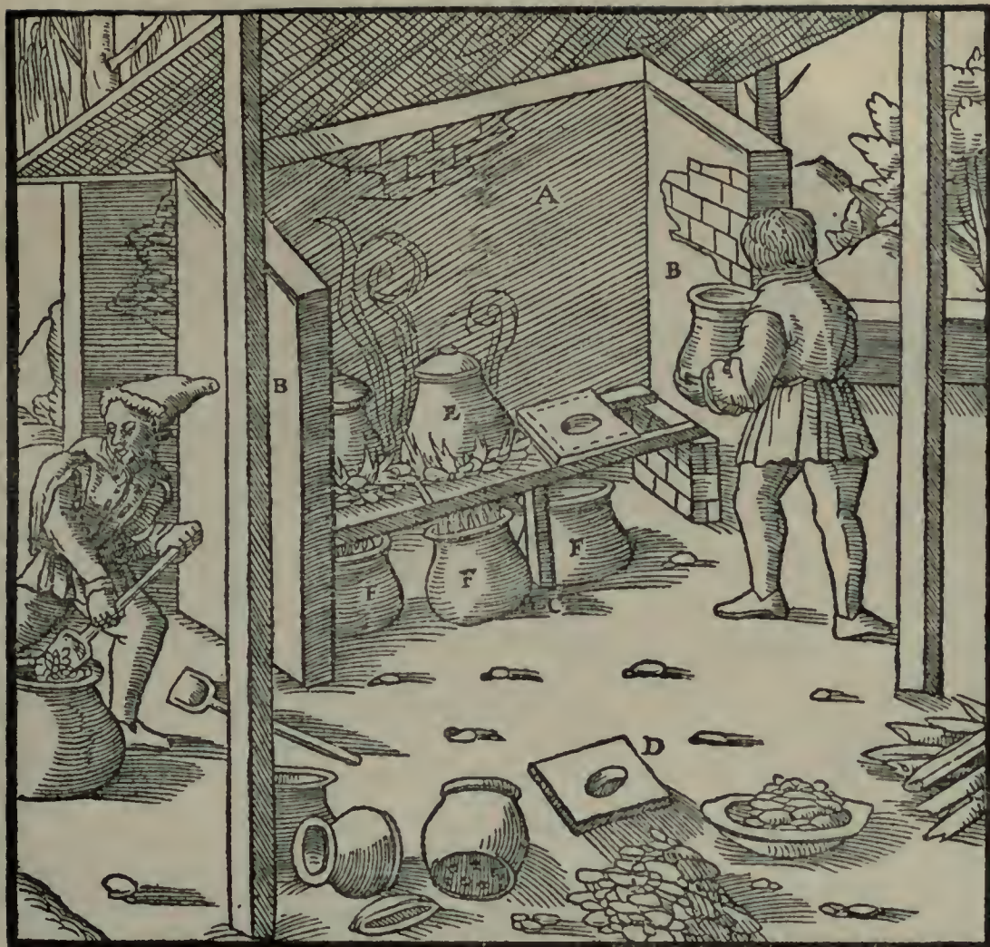
A—LONG WALL. B—HIGH WALLS. C—LOW WALLS. D—PLATES. E—UPPER POTS. F—LOWER POTS.
