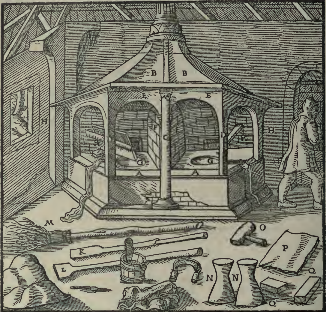
A—HEARTH OF THE FURNACE. B—CHIMNEY. C—COMMON PILLAR. D—OTHER PILLARS. THE PARTITION WALL IS BEHIND THE COMMON PILLAR AND NOT TO BE SEEN. E—ARCHES. F—LITTLE WALLS WHICH PROTECT THE PARTITION WALL FROM INJURY BY THE FIRE. G—CRUCIBLES. H—SECOND LONG WALL. I—DOOR. K—SPATULA. L—THE OTHER SPATULA. M—THE BROOM IN WHICH IS INSERTED A STICK. N—PESTLES. O—WOODEN MALLET. P—PLATE. Q—STONES. R—IRON ROD.
