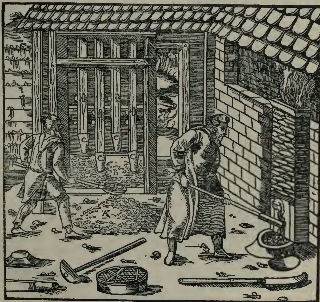
A—CHARCOAL. B—MORTAR-BOX. C—STAMPS.
