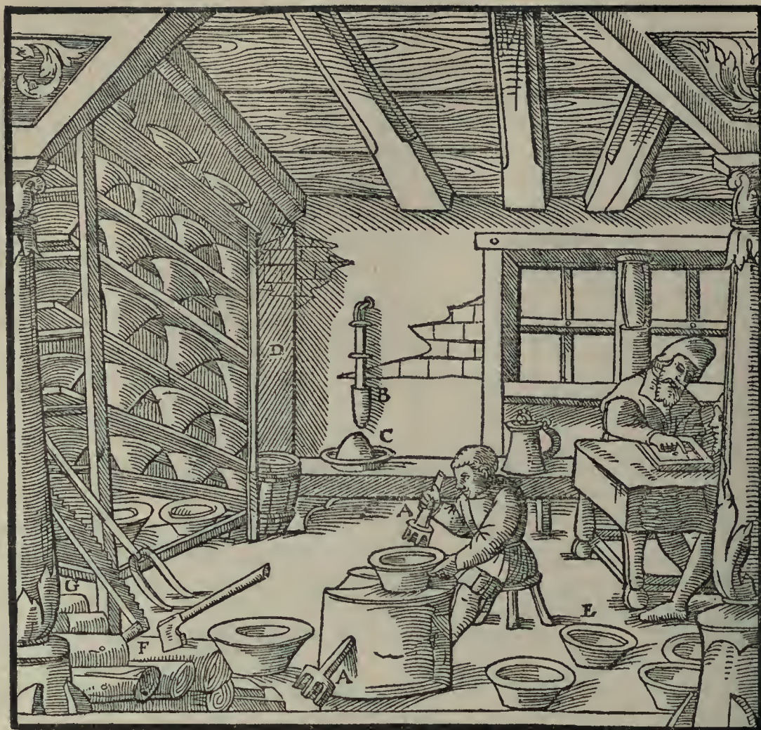
A—PESTLE WITH TEETH. B—PESTLE WITHOUT TEETH. C—DISH OR TRAY FULL OF ASHES. D—PREPARED TESTS PLACED ON BOARDS OR SHELVES. E—EMPTY TESTS. F—WOOD. G—SAW.
