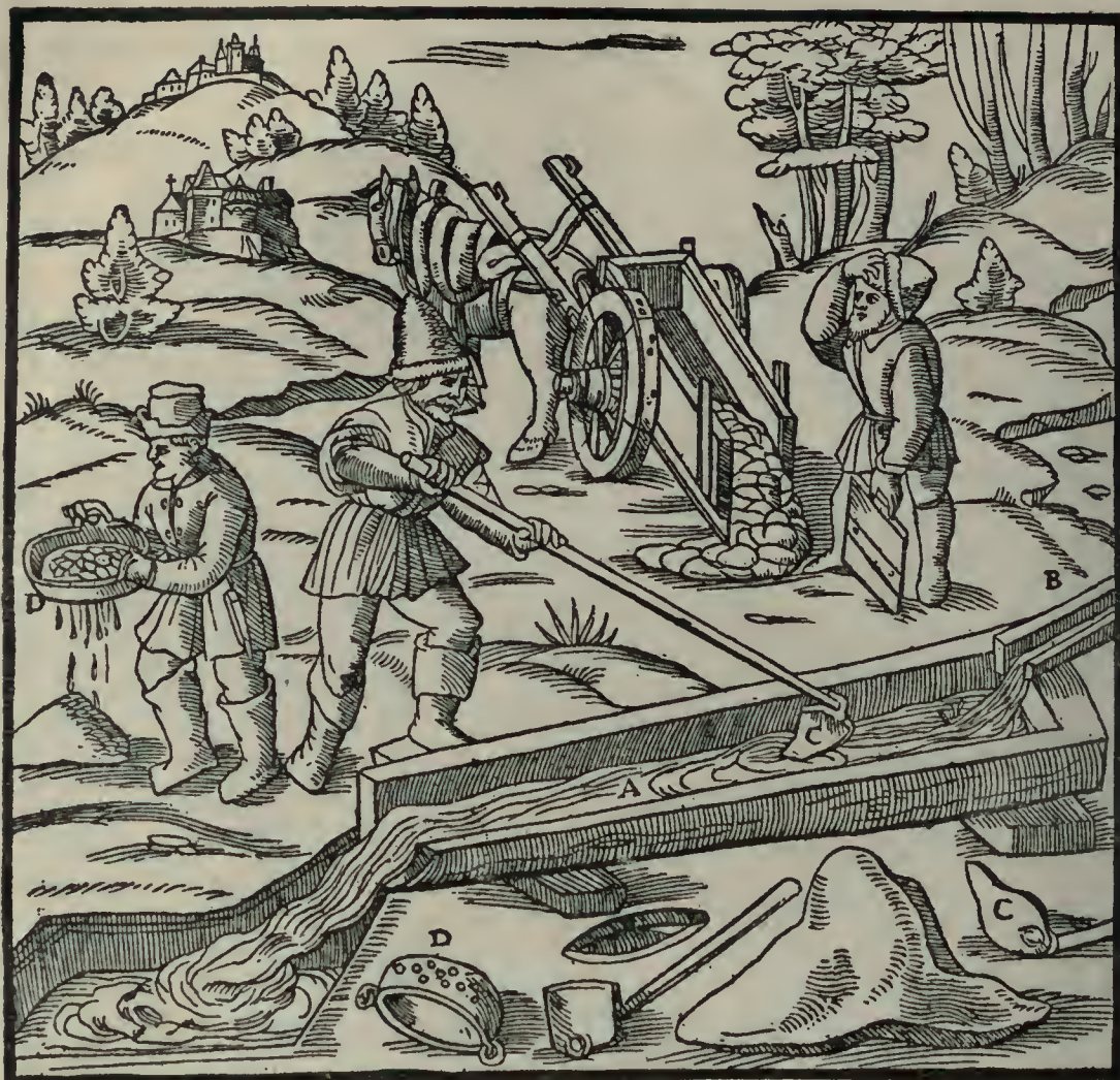
A—TROUGH. B—LAUNDER. C—HOE. D—SIEVE.
