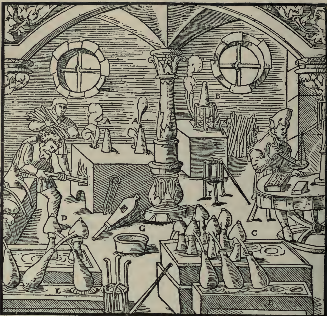
A—AMPULLAE ARRANGED IN THE VESSELS. B—AN AMPULLA STANDING UPRIGHT BETWEEN IRON RODS. C—AMPULLAE PLACED IN THE SAND WHICH IS CONTAINED IN A BOX, THE SPOUTS OF WHICH REACH FROM THE OPERCULA INTO AMPULLAE PLACED UNDER THEM. D—AMPULLAE LIKEWISE PLACED IN SAND WHICH IS CONTAINED IN A BOX, OF WHICH THE SPOUT FROM THE OPERCULA EXTENDS CROSSWISE INTO AMPULLAE PLACED UNDER THEM. E—OTHER AMPULLAE RECEIVING THE DISTILLED aqua AND LIKEWISE ARRANGED IN SAND CONTAINED IN THE LOWER BOXES. F—IRON TRIPOD, IN WHICH THE AMPULLA IS USUALLY PLACED WHEN THERE ARE NOT MANY PARTICLES OF GOLD TO BE PARTED FROM THE SILVER. G—VESSEL.
