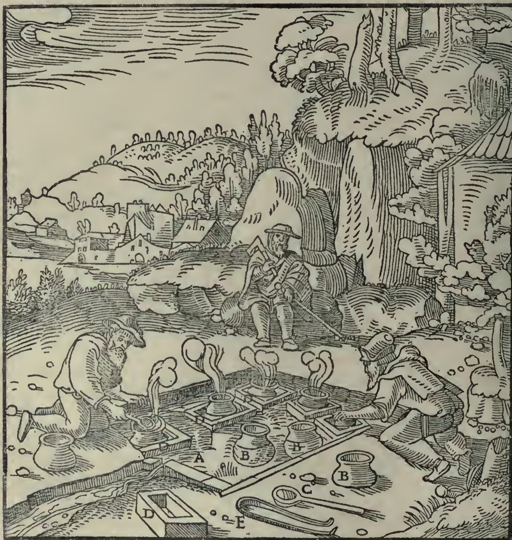
A—POOL. B—POTS. C—LADLE. D—PANS. E—TONGS.
