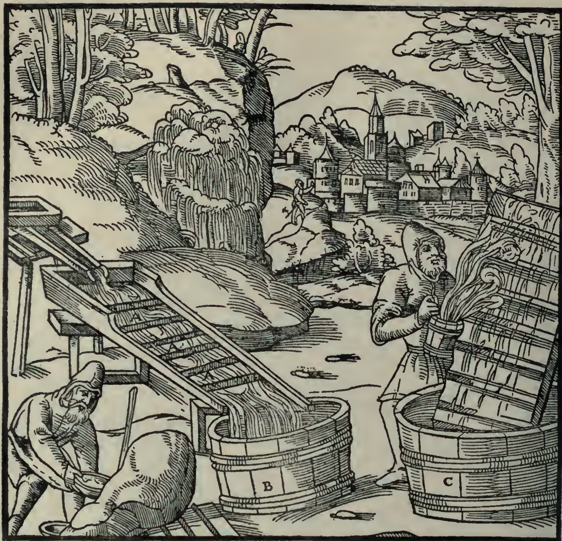
A—CROSS GROOVES. B—TUB SET UNDER THE SLUICE. C—ANOTHER TUB.
