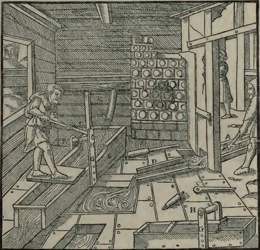
A—FIRST LAUNDER. B—THREE-TOOTHED RAKE. C—SMALL SETTLING PIT. D—LARGE BUDDLE. E—BUDDLE RESEMBLING THE SIMPLE BUDDLE. F—SMALL ROLLER. G—BOARDS. H—THEIR HOLES. I—SHOVEL. K—BUILDING. L—STOVE. (THIS PICTURE DOES NOT ENTIRELY AGREE WITH THE TEXT).
