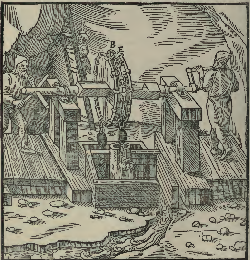
A—AXLE. B—DRUM. C—DRAWING-CHAIN. D—BALLS. E—CLAMPS.
