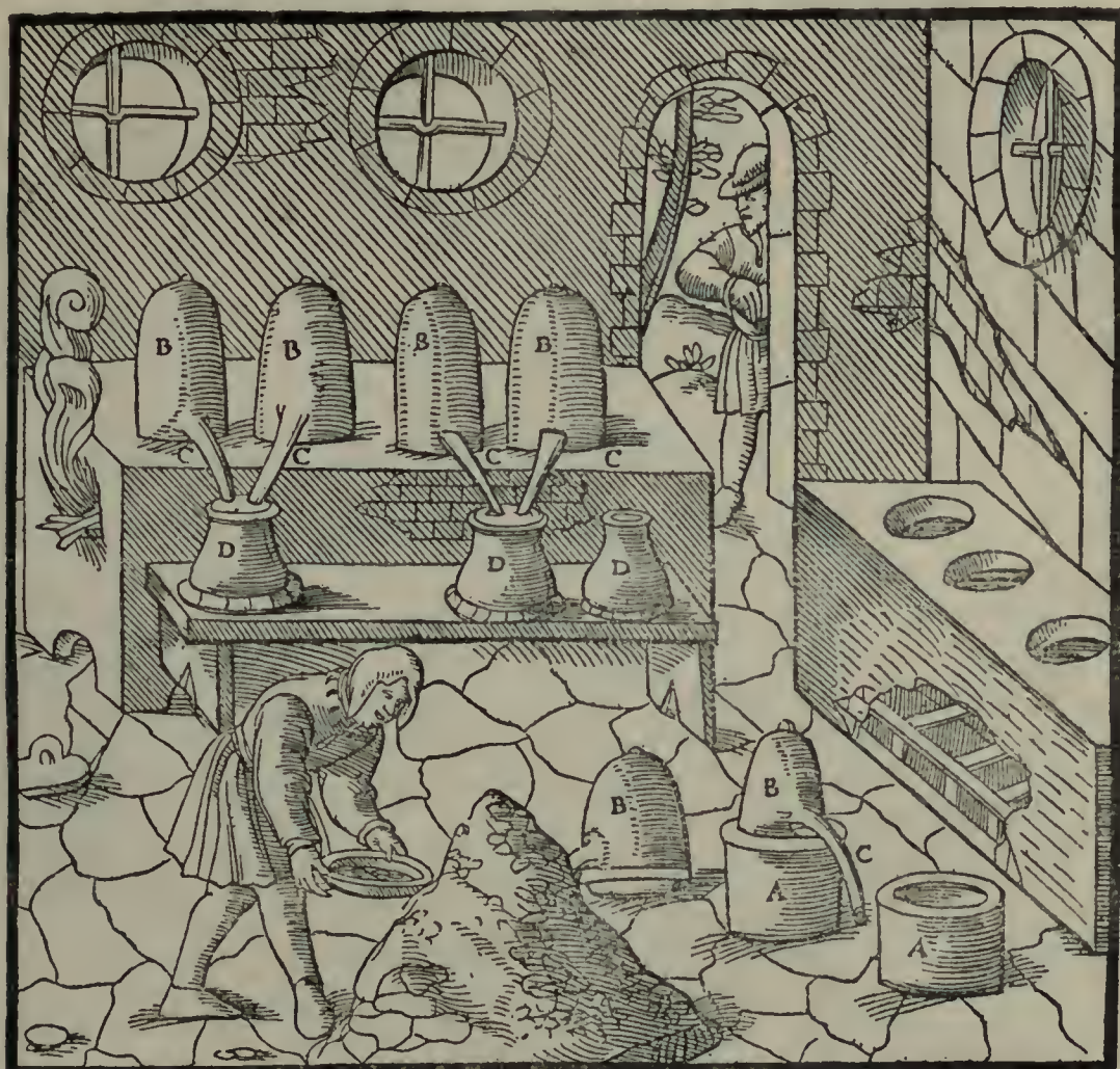
A—POTS. B—OPERCULA. C—NOZZLES. D—GOURD-SHAPED EARTHENWARE VESSELS.
