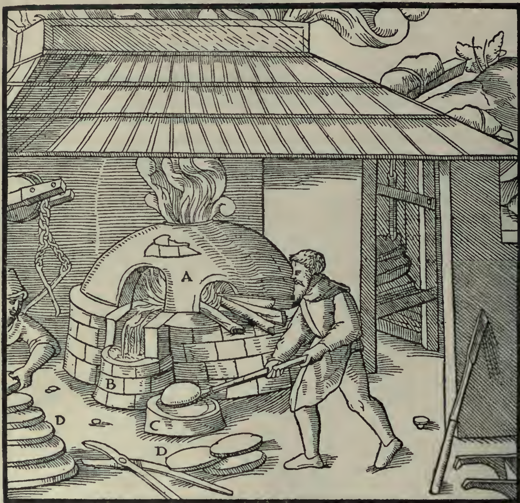
A—FURNACE. B—FOREHEARTH. C—DIPPING-POT. D—CAKES.
