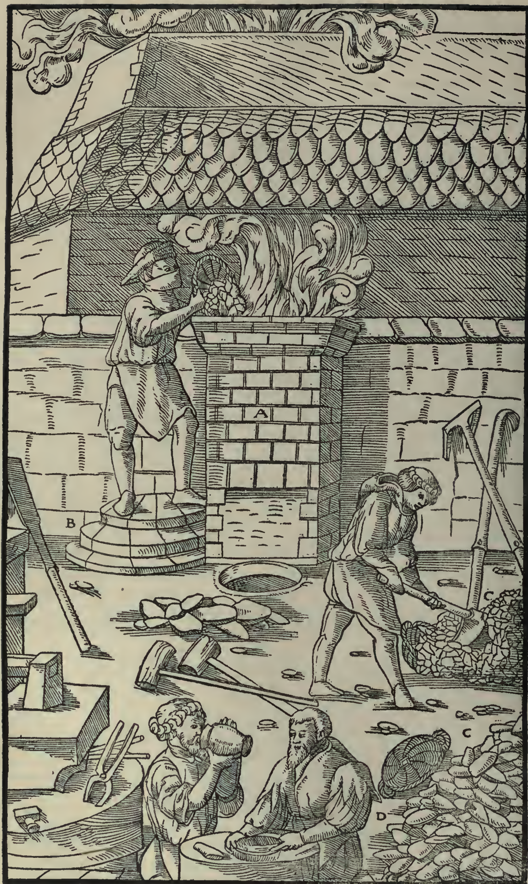
A—FURNACE. B—STAIRS. C—ORE. D—CHARCOAL.
