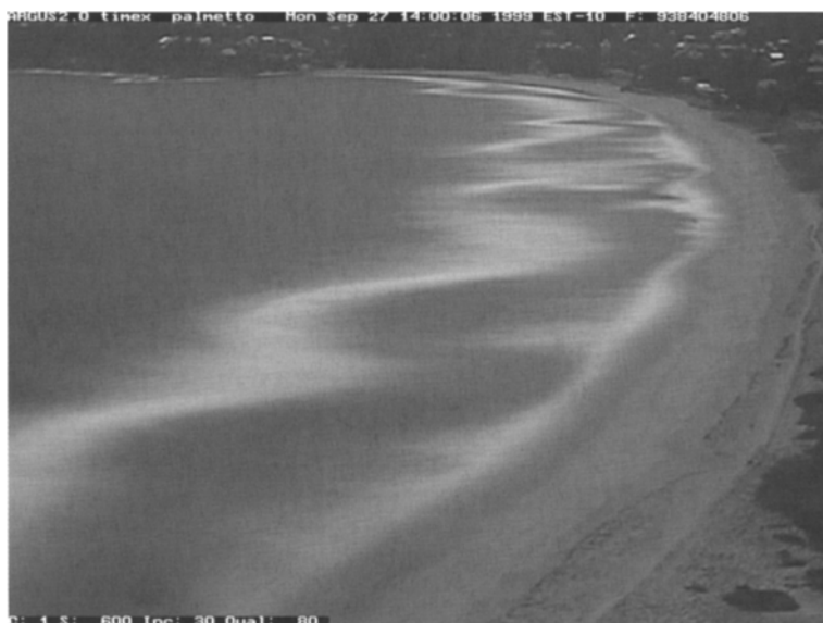
Figure 3. Time lapse image showing wave breaking positions at Palm Beach, Sydney (from the Argus Camera managed by G. Symonds).
