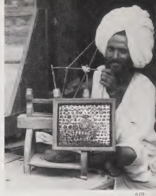
610. Delhi. Late 19th century A seal carver at the Dariba Bazaar, Delhi, sits behind his weighted carving lathe before which, to illustrate his skill, is a framed paper bearing imprints of seals he has made. The Delhi sealstone carvers were the most famous in India because of their skill in making highly aesthetic calligraphic Persian and Urdu inscriptions in Arabic characters. Collection the author, Porvoo
