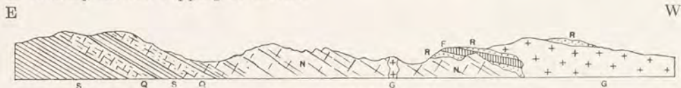
Fig. 27. Generalized Section across the Bushveld Igneous Complex in the Eastern Transvaal. S. Shales (Pretoria Series). Q. Magaliesberg Quartzite (Pretoria Series). N. Norit, Pyroxenite, etc. G. Red or Bushveld Granite. R. Quartzites etc., (Rooiberg Series). F. Felsites, etc. Length of Section: 30 miles (48 km).
