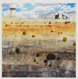
The Koffiefontein Mine sidewall illustrates the different strata penetrated by the kimberlite pipe that was mined there.
