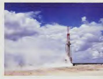
Drilling of an alluvial target to establish the presence and thickness of potentially diamondiferous gravel.
