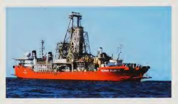
A Debmar vessel used for mining the sea-bed gravel for its diamonds.
