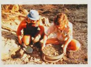
Ashton Joint Venture samplers collecting wash from a dry riverbed to check for kimberlite indicator minerals.
