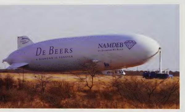
Zeppelins or blimps or dirigibles are suitable for some forms of airborne geophysical surveys, being less susceptible to turbulence than conventional aircraft.
