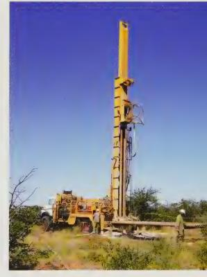
Drilling a kimberlite pipe in Botswana.
