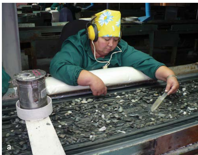
Fig. 1.5 a and b Conveyor belts for sorting emerald in the mineral processing plant at the Malysheva Mine. Photographs by L. Kiefert in 2007.
