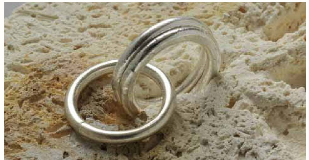
The kiln brick makes fused chain easy; just dig a small channel to support the two closed rings on either side of your active ring. Pile up extra links on the brick as your chain grows.
