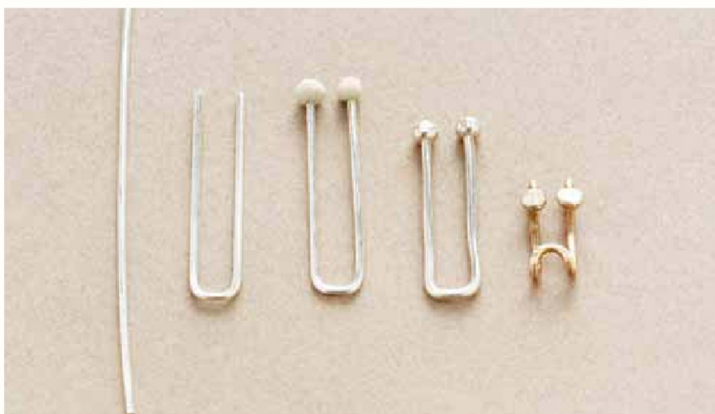
Ball-end clasps in the different stages of forming, left to right : the straight, cut wire; the speared fresh clay ends; the fired clasp; and one that has been bent both top and bottom to fit a very small piece of beadwork.
