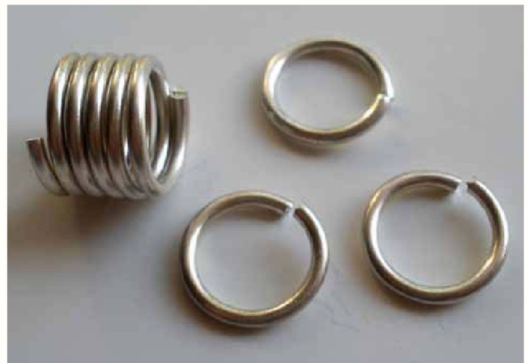
Jump rings cut from 14-gauge fine silver wire.
