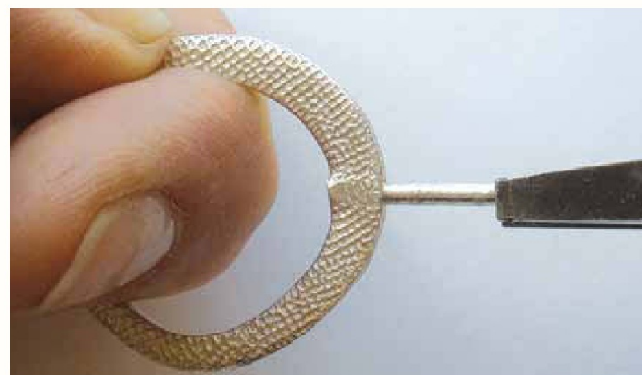
Straightening and work-hardening a rivet post: Use nylon-jaw pliers for straightening any gauge of wire and flat-nose pliers to get a good grip on the end of the wire, in preparation for twisting it a quarter to a full turn to harden the post.
