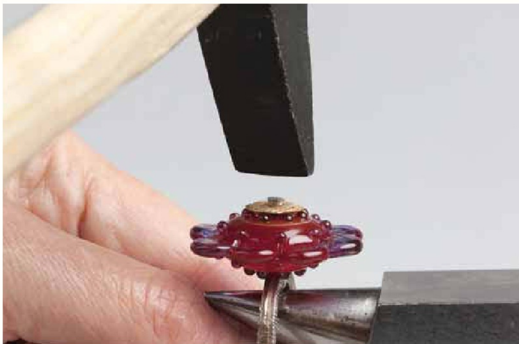
A shorter rivet wire being tapped with the chisel point of the riveting hammer to spread the top of the wire enough to trap the bead and the fine silver rivet angel but still allow the bead to spin. (Bead by Sarah Moran.)
