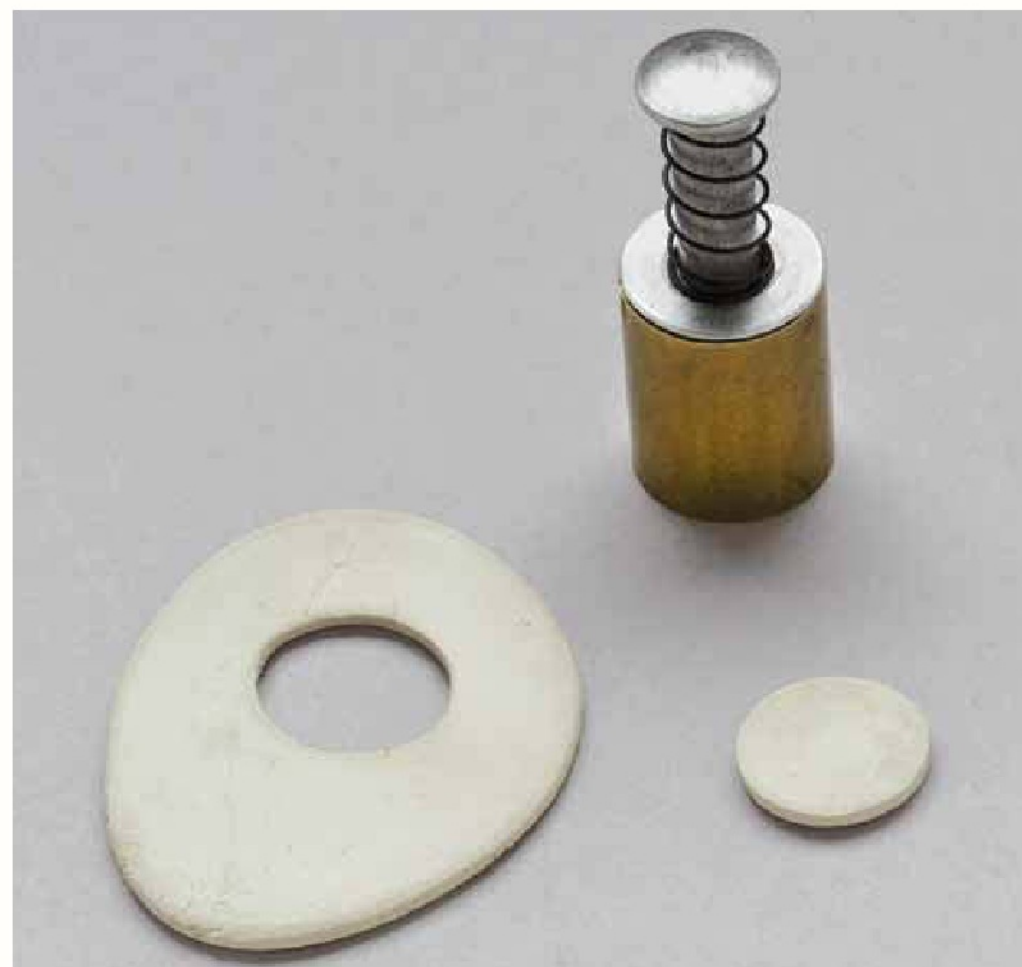
A simple circle, cut out of a rolled sheet of metal clay.
