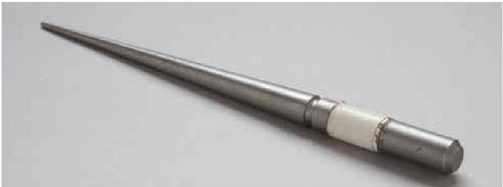
A slender bezel mandrel, useful for forming bezels, graduated coils, or for supporting small chain links in the work-hardening process.
