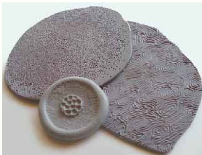
Texture sheets made from two-part silicone molding compound.
