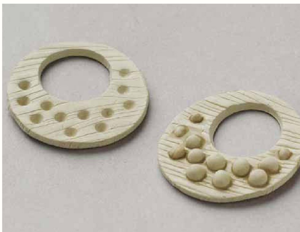
Smoothly rolled and dried balls of fine silver metal clay are placed in wetted divots, to seat them snugly in place. The finished, fired balls can be left round or hammered.
