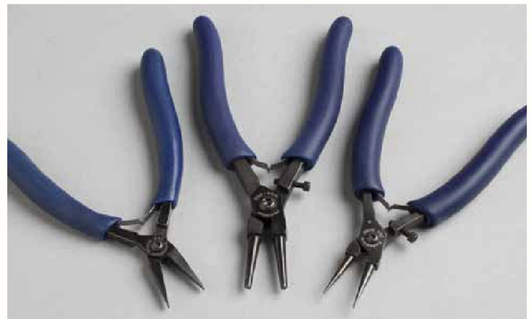
Three workhorse pliers from Swanstrom: a flat-nose ( left ), a heavy-duty round-nose ( middle ), and a regular round-nose ( right ). These are my favorite pliers on the market.
