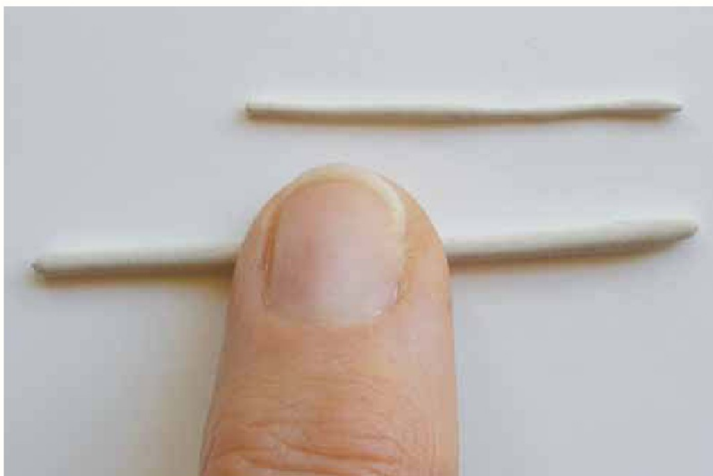
It's easy to roll snakes of metal clay with your fingertips to make toggle bars or tiny little snakes to reinforce box joins.
