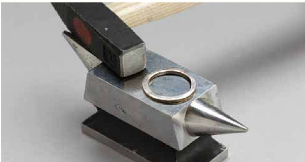
I use the chasing side of my riveting hammer for forging, hardening, and most general-purpose hammering.
