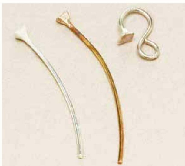
Sculptural S-hooks in various stages: cut wire with drying clay tip; the fired and patinated ornamented wire before bending; and a finished, formed hook.
