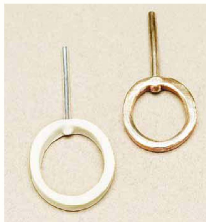
A fresh greenware clay ring and a fired, finished version ready for riveting. Remember that the ring will shrink about 15% in the firing!
