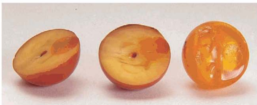
Figure 1.20 Baltic amber, broken bead showing surface effect of heat treatment.
