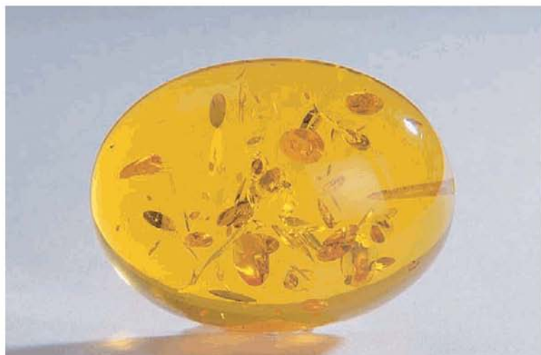
Figure 1.23 Plastic simulant with imitation stress fractures.
