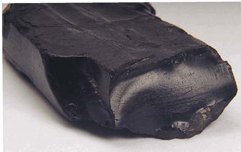
Figure 2.2 Piece of Whitby jet showing conchoidal fracture.
