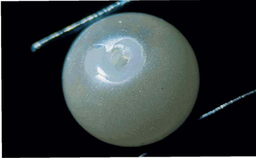
Figure 9.21 Coated plastic bead showing surface wear around drill hole.
