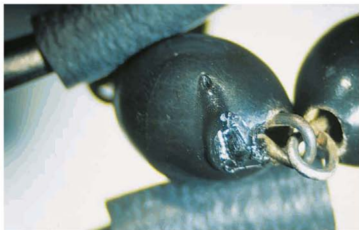
Figure 2.12 Jet simulant bead, showing excessive damage from hot-point test.
