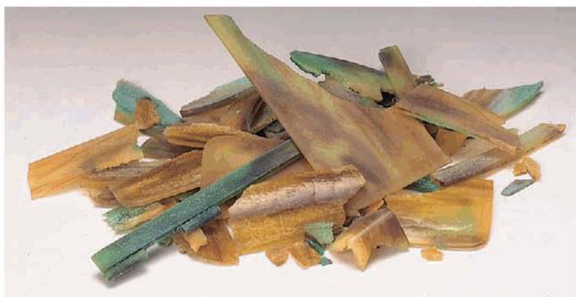
Figure 13.3 Degraded celluloid box that once imitated tortoiseshell.
