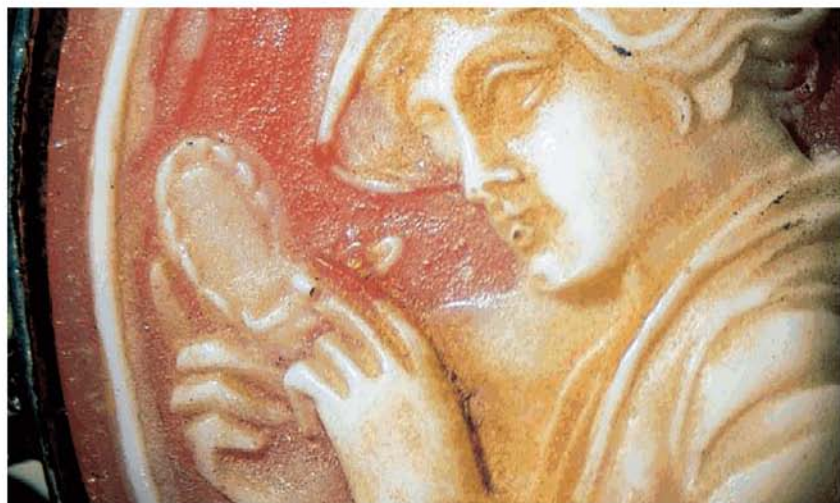
Figure 10.19 Detail of a plastic cameo, showing signs of moulding.
