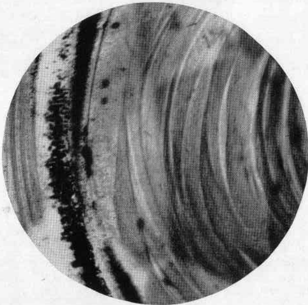
Figure 4 synthetic ruby of early production. Strongly curved and well-marked stria- tions and dense cloud of gas bubbles placed along striae.
