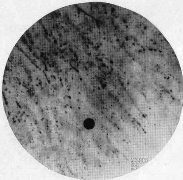
Figure 1 synthetic sapphire Dense cloud of minute spherical gas bubbles, some elongated wormlike gaseous inclusions and one very large gas bubble.
