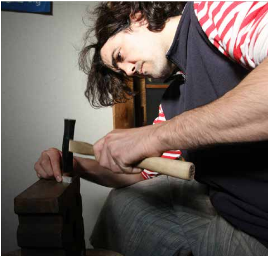
One of the authors, Jaume Labro, forging a metal billet of mokume-gane. Photo courtesy of Jaume Labro.
