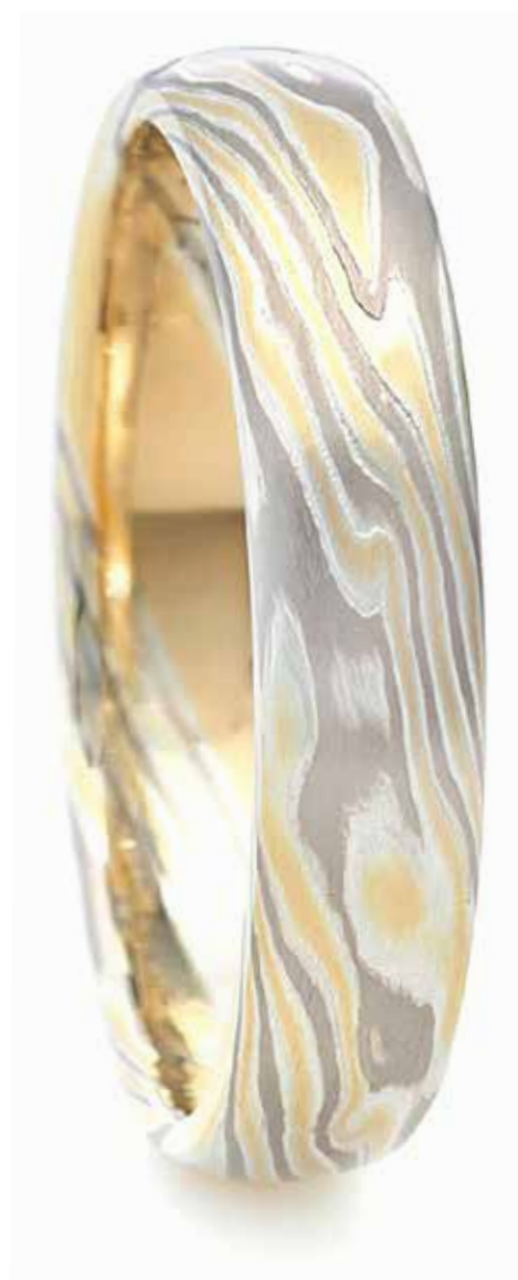
A wedding ring of 18K white and yellow gold and silver (right), made by Jaume Labro using mokume-gane, with a close-up of the finished pattern (above). Photo by Jaume Labro.
