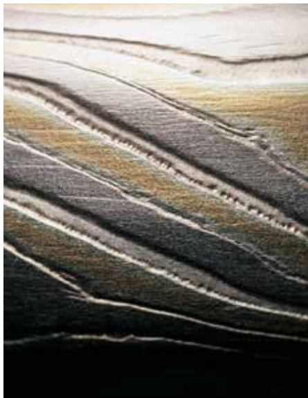
A wedding ring of 18K white and yellow gold and silver (right), made by Jaume Labro using mokume-gane, with a close-up of the finished pattern (above). Photo by Jaume Labro.
