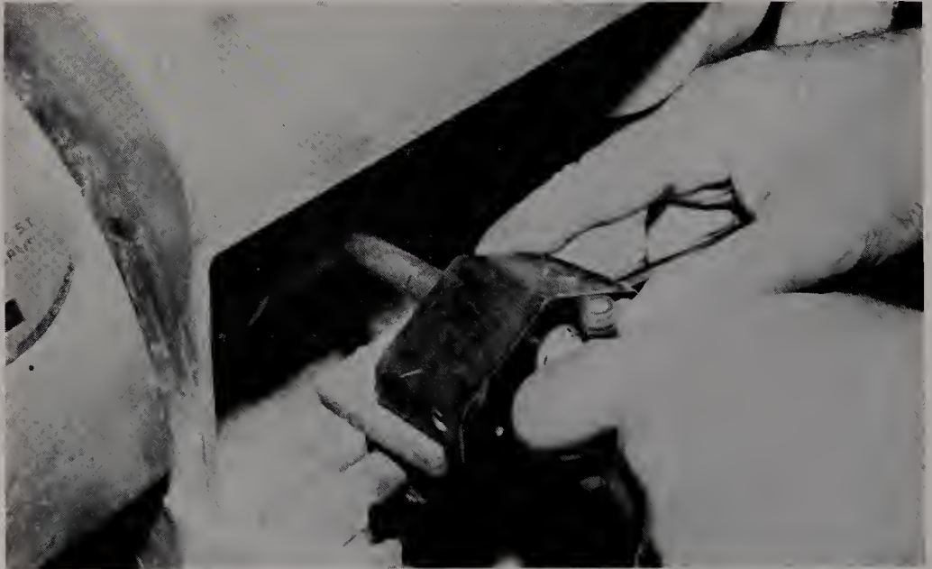
The diamond dresser is applied either held by hand or in jig, resting on tool rest. The diamond or diamonds should touch the grinding wheel just below an imaginary horizontal line drawn through its center.
