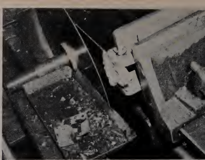
A slab grabber is used to hold odd-shaped material and is, in turn, held in the vise of the slab saw.
