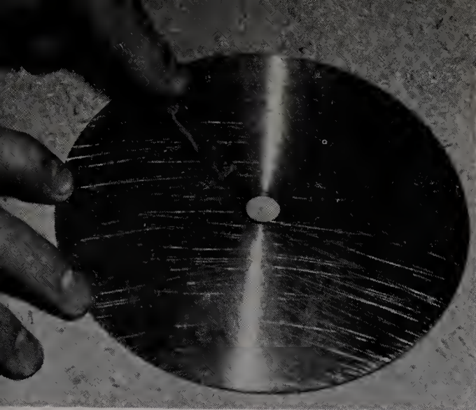
A broken hacksaw blade is a good tool for scoring a lap. Scores should run in all directions.
