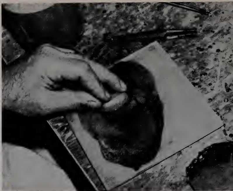
A flat surface can be achieved by using a mixture of water and carborundum grit on a glass plate. The whole surface of the glass should be used.
