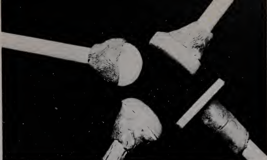
Some mistakes in doping. From left to right (clockwise): (1) doping wax hides out-line of stone; (2) the stone is off-center; (3) the doping wax does not support the stone sufficiently; (4) the stone is not mounted at right angles to dop stick.
