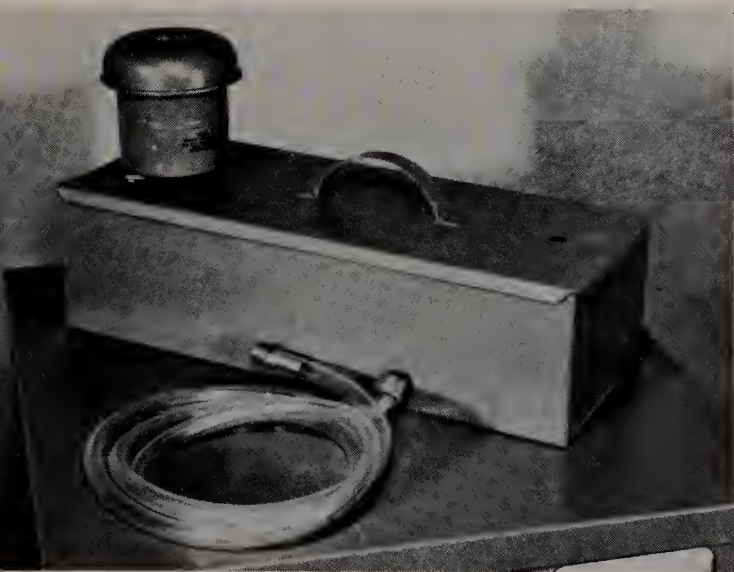
The best way to supply water, particularly for the grinding operation, is a circulating pump.
