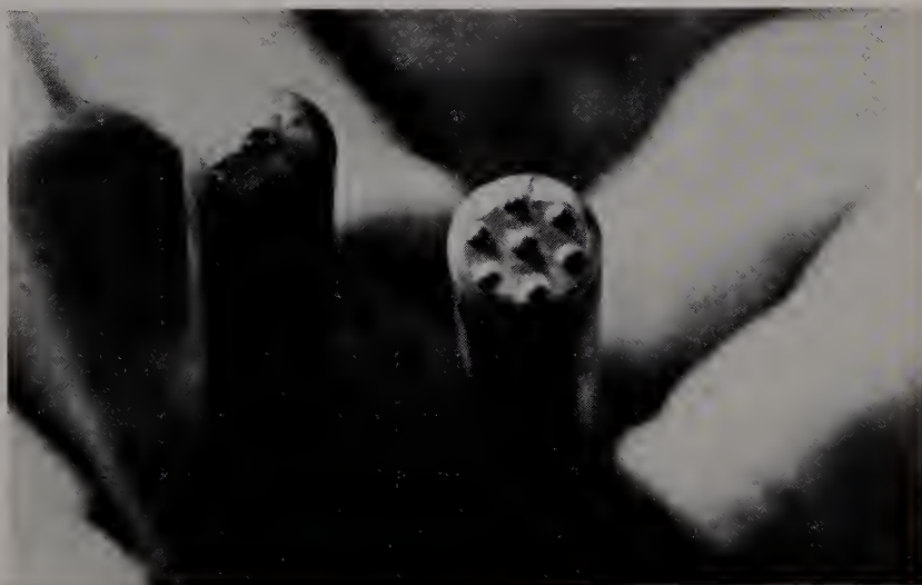
Diamond wheel dressers come set with one piece of diamond or with many small diamond chips. The one-stone dresser is really all that is needed. The multiple-diamond dresser is good for producing a really smooth surface.
