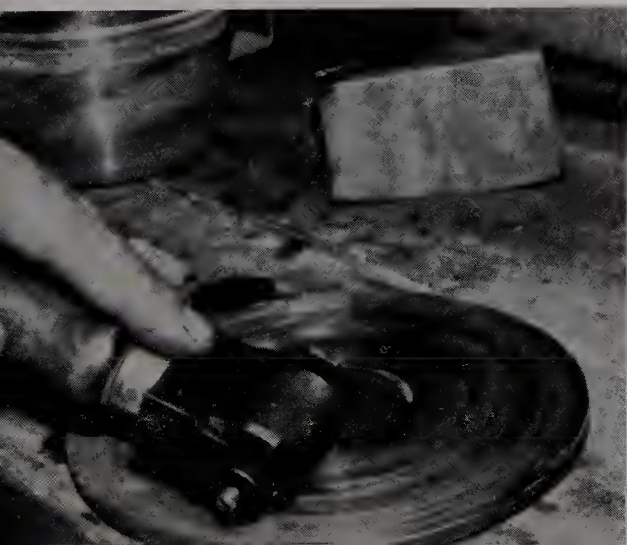
A steel roller is used to push the diamond particles into the metal.
