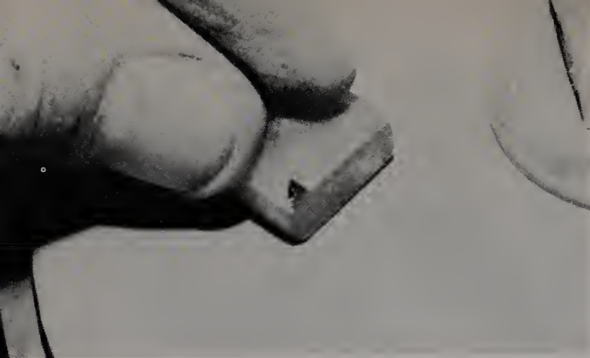
To smooth the table, the stone is best held by hand.
