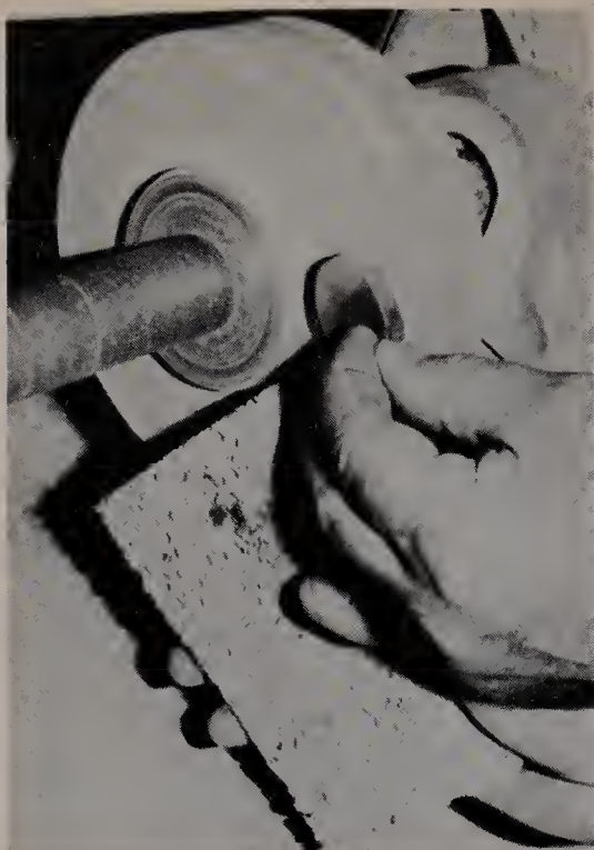
A flat surface can be trued on the side of the grinding wheel. Water must be supplied by a sponge held in one hand.
