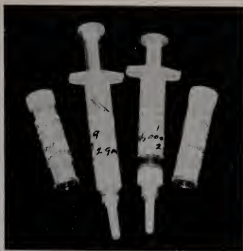
Diamond for charging comes as dry powder in plastic vials or mixed with a carrying agent in small plastic syringes.
