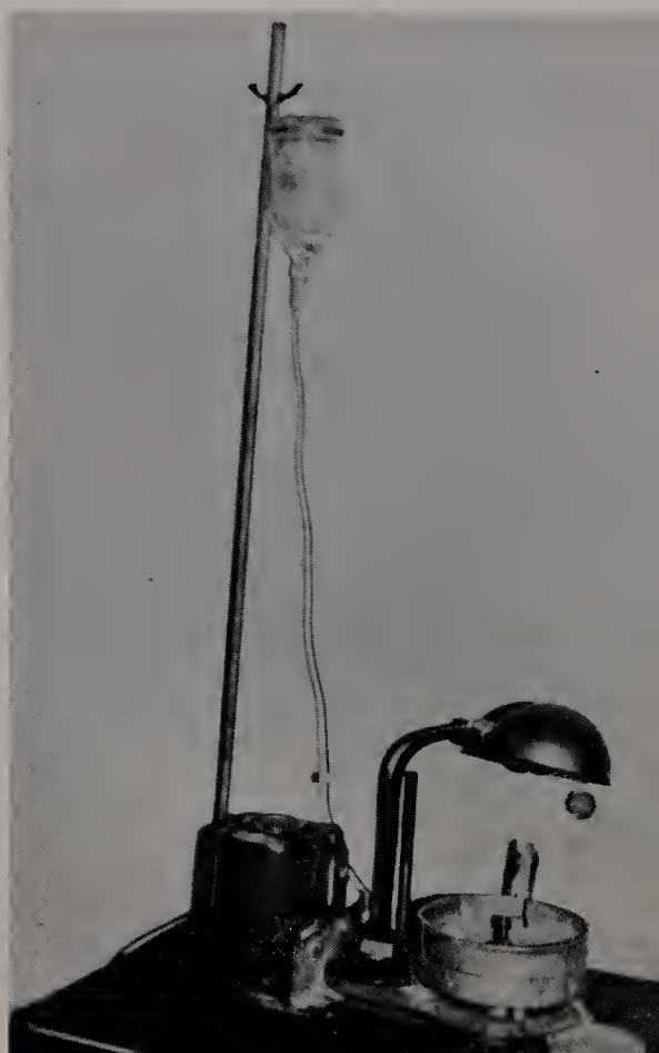
A transfusion bottle is a good source of water supply, particularly for faceting operations.
