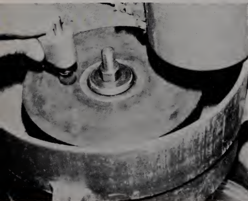
Lee Manufacturing recently brought out a 90° dop holder for grinding and polishing the table of faceted stones.
