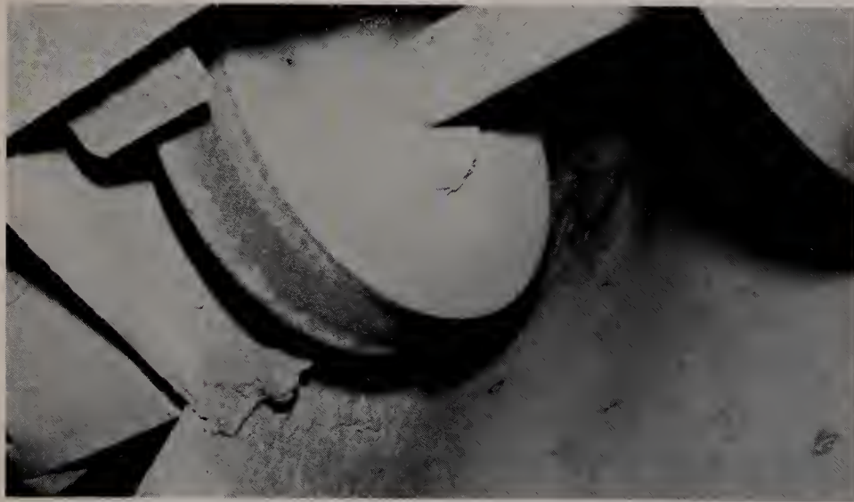
Shown here is a badly deformed wheel in need of "dressing."
