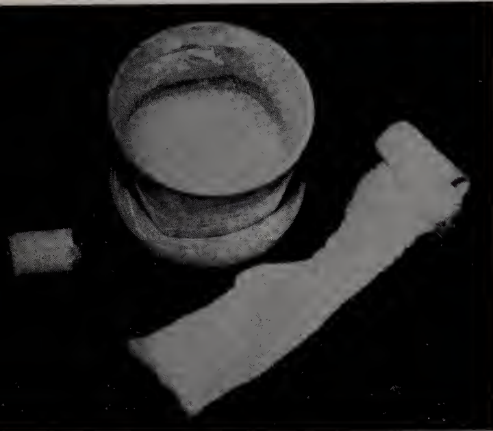
Polishing powders may be applied with pads made from rolled-up linen strips.
