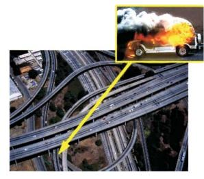
**Figure 2.13** Systems such as OnStar allow information on the location of an accident, determined by a GPS unit in the vehicle, to be sent to a central office and compared to a GIS database of highways and streets, to determine the incident location so that emergency teams can respond
