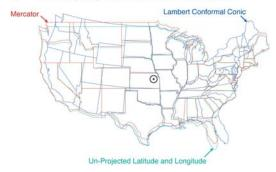
**Figure 5.14** (A) The so-called *unprojected* or Plate Carrée projection, a tangent cylindrical projection formed by using longitude as x and latitude as y. (B) A comparison of three familiar projections of the USA. The Lambert Conformal Conic is the one most often encountered when the USA is projected alone, and is the only one of the three to curve the parallels of latitude, including the northern border on the 49th Parallel (Reproduced by permission of Peter H. Dana)
