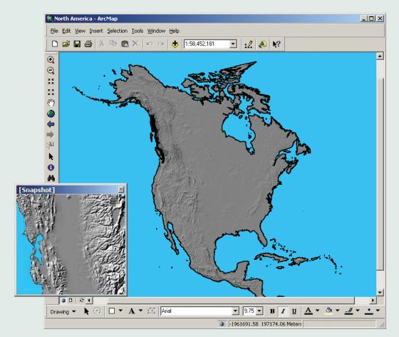
**Figure 8.6** Shaded digital elevation model of North America used for comparison of image compression techniques in Table 8.2. Original image is 8726 by 10618 pixels, 8 bits per pixel. The inset shows part of the image at a zoom factor of 1000 for the San Francisco Bay area
