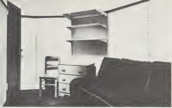
179 Interior of Twin Deployment Unit. The large cylinder in daytime functioned as a 20-foot living-kitchen room. Note the plug-in electrical strip forming entire circle around interior of the dwelling unit at head of keyhole strips. Electrical appliances could be plugged into the strip at any point.
