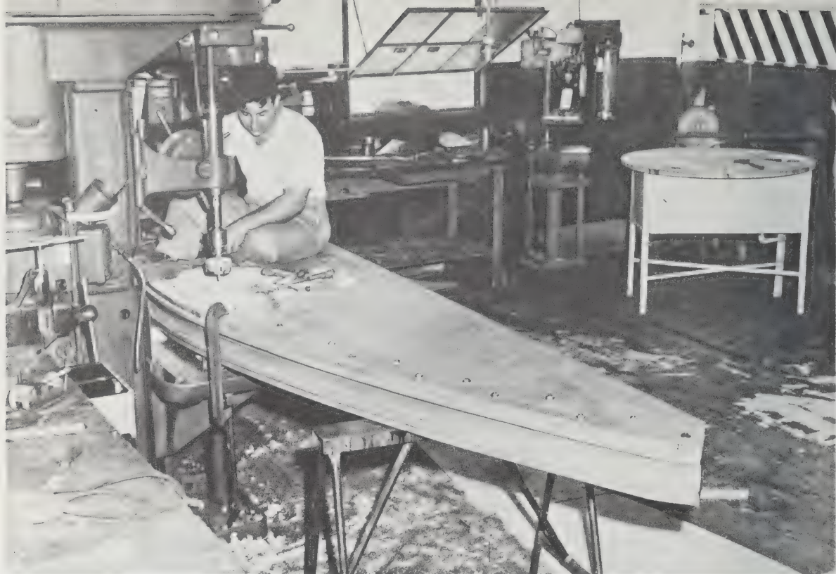
204 Only those tools unique to the aircraft industry are shown in this series. Shown is the wood die, a typical aircraft industry soft tool, used for the forming of roof ribs of the Dymaxion dwelling machine.
