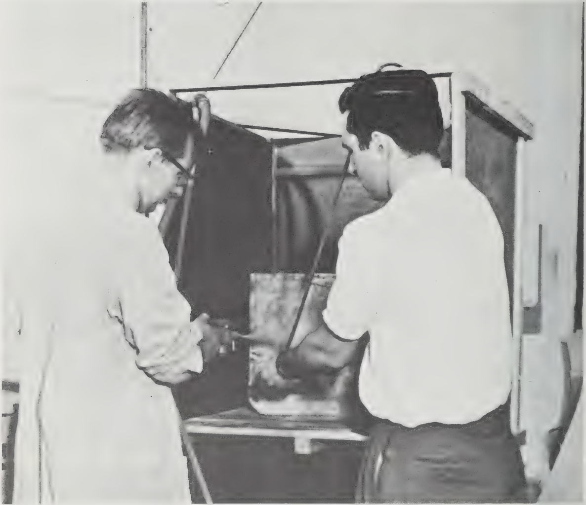
92 Research students at the Institute of Design, Chicago, in 1948 testing the Fog Gun. (Subsequent experiments were conducted at Yale and other universities.) A one-hour massaging pressure bath used only a pint of water. If fog gun bathing were done in front of a heat lamp, all the sanitary and muscle-relaxing effects of other types of bathing could be effected without the use of any bathroom. Since there were no run-off waters, tons of plumbing and enclosing walls could be eliminated, and bathing would become as much an "in-the-bedroom" process as dressing. Fuller holds that the other functions of the bathroom may be effected by odorless, dry-packaging machinery, employing modern plastics, electronic sealing, dry-conveying systems.
