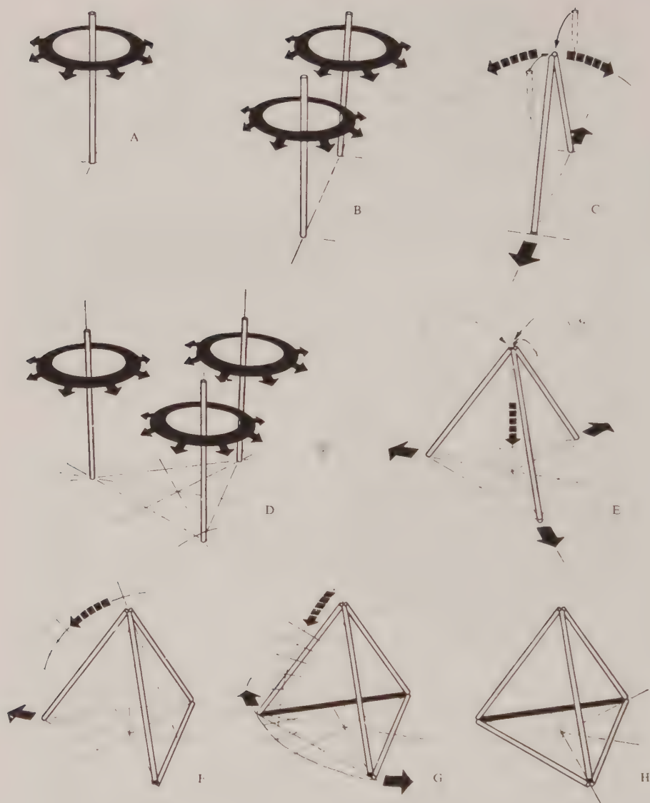
Fig. 621.10 Falling Sticks: Six Vectors Provide Minimum Stability:
