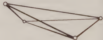
A fully stabilized square is actually a "shallow" tetrahedron
