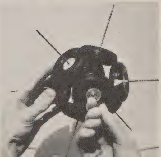
Fig. 465.10 The vector equilibrium with wheels showing that when one wheel is immobilized (the lower wheel in photos) and the system is rotated about the axis shared by the fixed wheel and its opposite wheel, the opposite wheel remains stationary but the other six wheels rotate in concert. The polarity of the system is thus demonstrated.
