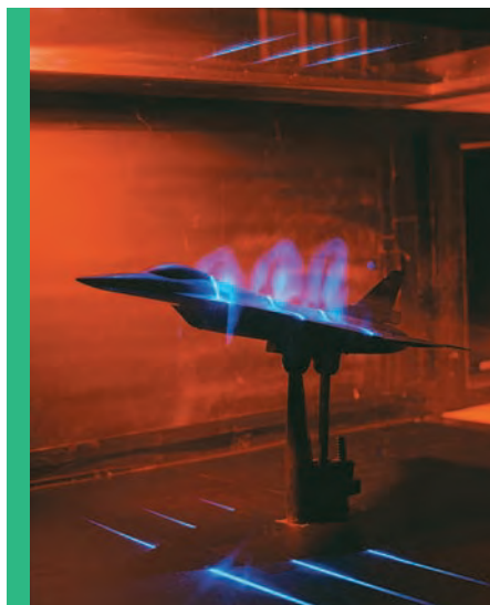
NASA researchers visualize the airflow around this model jet with smoke illuminated by a laser light sheet. ( NASA/Langley Research Center )
