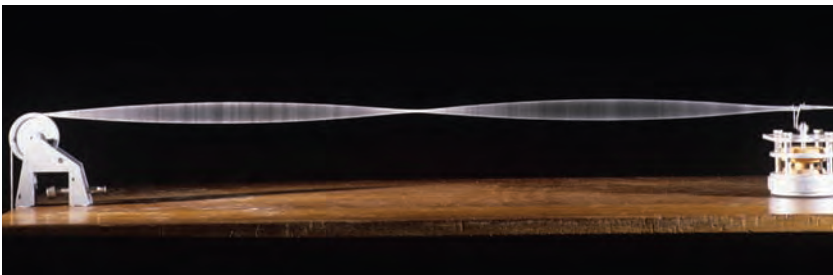
A string vibrating at twice the lowest frequency—note the stationary point in the middle ( Andrew Lambert Photography/Photo Researchers, Inc. )
