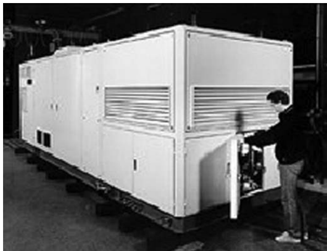
FIGURE 8.10 A 250 kW Ballard Power Systems Fuel Cell with a Built-In Natural Gas Reformer
