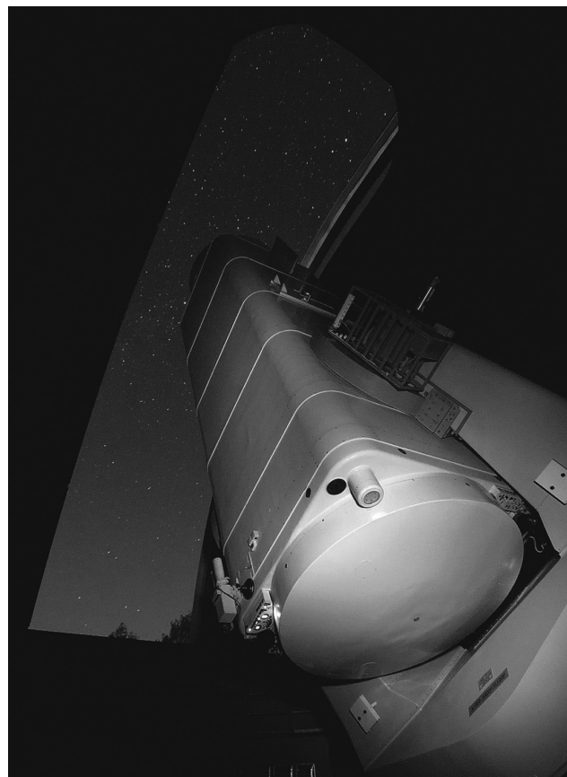
The 2-meter Zeiss reflector of the Thüringer Landessternwarte "Karl Schwarzschild" in Jena-Tautenburg, Germany. This is the world's largest Schmidt telescope. Schmidt telescopes use a spherical mirror in combination with a correction lens.
