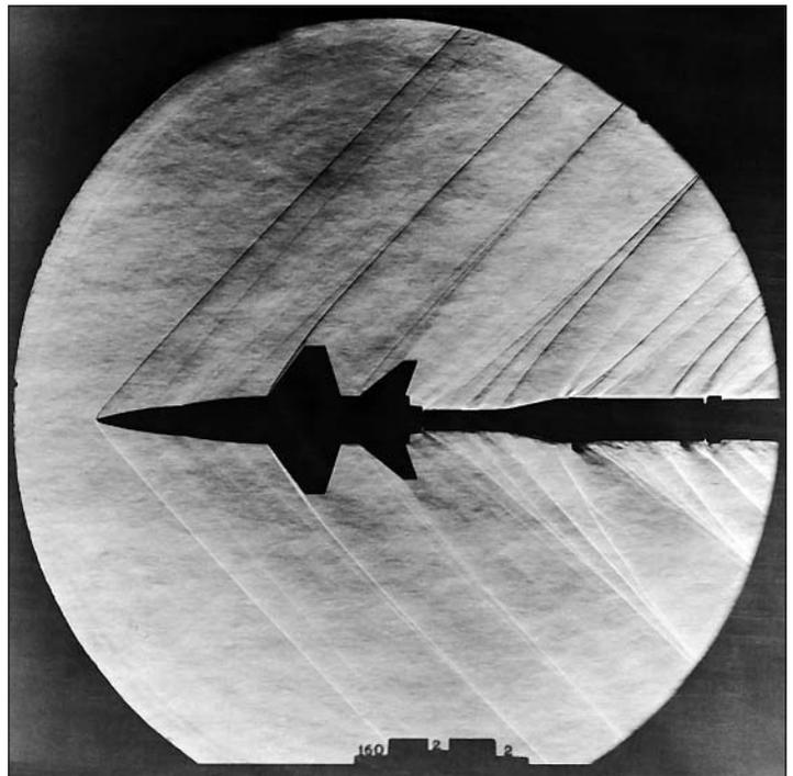
*The shock waves caused by supersonic flight can be seen emanating from a model of the X-15 as it flies through a supersonic pressure tunnel. (NASA)*
