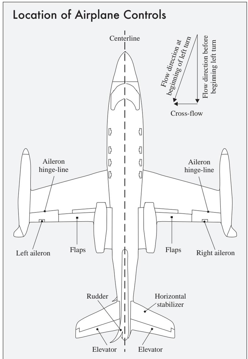
vator is deflected to change the pitch angle of the airplane: When the trailing edge of the elevator is moved upward, a down force is generated on the horizontal stabilizer. The result is that the nose of the airplane pitches upward. The airplane will pitch in the opposite direction if the trailing edge of the elevator is moved downward.
