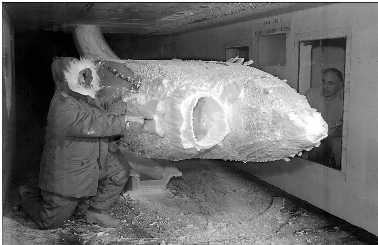
*The accumulation of ice on the exterior structures of an aircraft can affect a plane's lift and drag. NASA has conducted extensive research on icing in its icing research tunnel at the Glenn Research Center. (NASA)*
