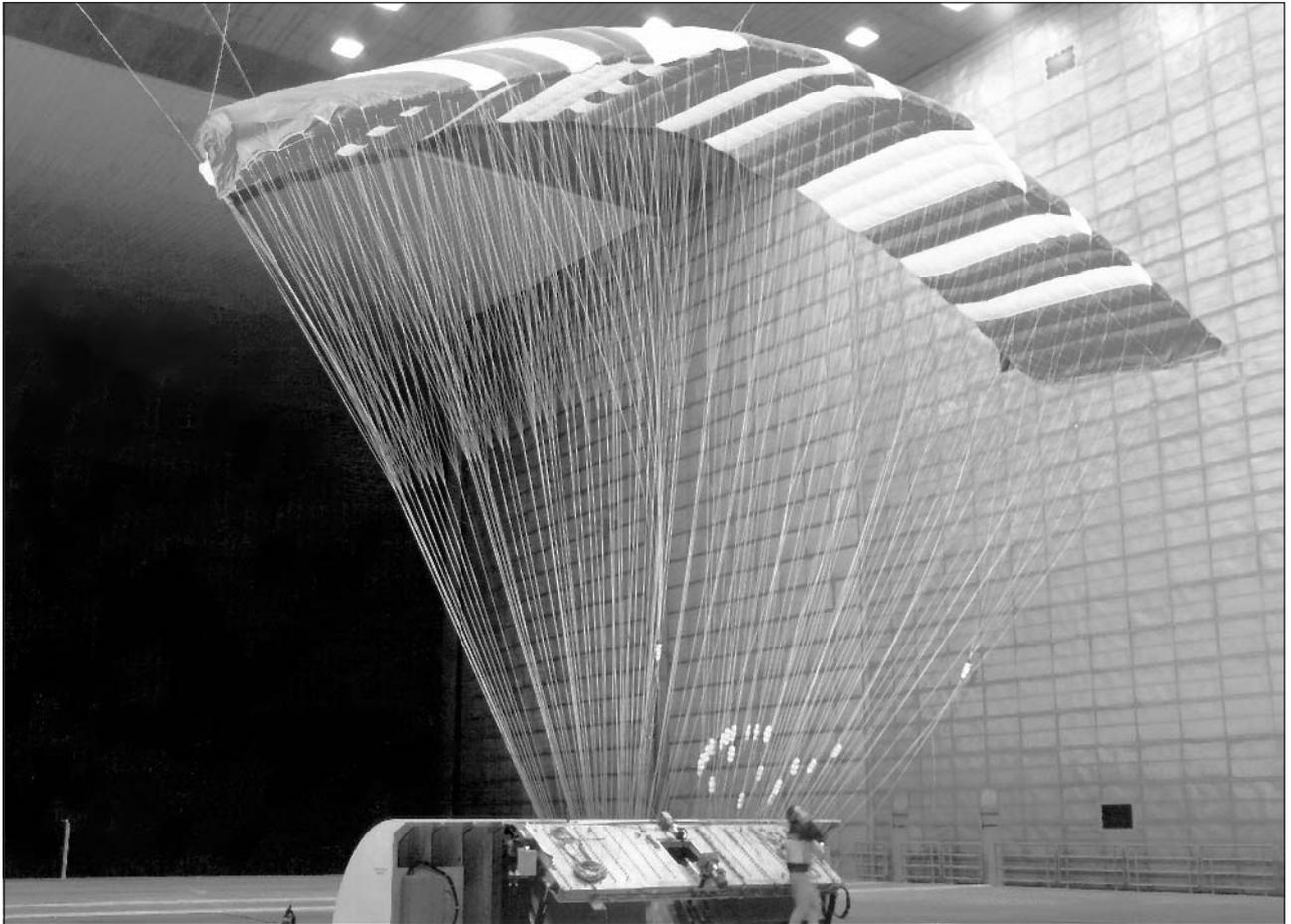
*NASA operates a number of wind tunnels for testing the designs of experimental aircraft. The world's largest wind tunnel is located at NASA's Ames Research Center in Mountain View, California, where this parafoil is being tested. (NASA)*
