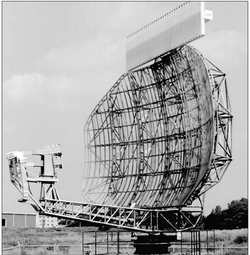
*A radar receiver locates objects and measures the distance to them by sending out short bursts of radio waves and measuring how long it takes for an echo of the bounced-back wave to return. (Raytheon Company)*
