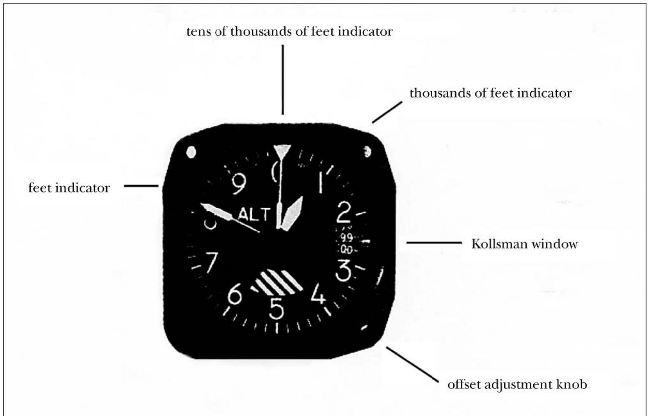
*An altimeter measures an aircraft's altitude in feet, thousands of feet, and tens of thousands of feet.*
