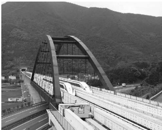
Fig. 8 Two Central Japan Railway MLX01 superconductor high-speed maglevs on test track in Yamanashi Prefecture.
