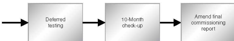
Fig. 5 Warranty period commissioning testing.
