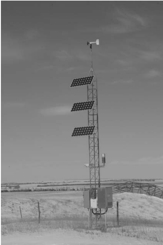
Fig. 11 A photovoltaic (PV)-powered instrumentation package near Gordon, Nebraska (Photo by Susan Ropp).
