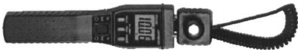
Fig. 7 A stick-type light meter with a retractable sensor. (Courtesy of Omega Inc.).
