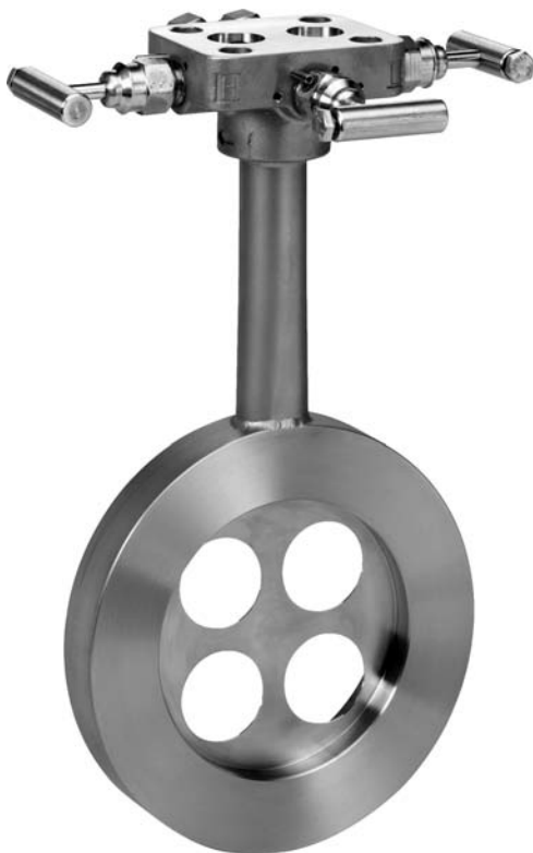
Fig. 3 Conditioning plate—compact orifice paddle-style plate (with integral manifold).
