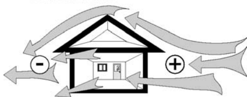
Fig. 10 Wind effect on houses.
