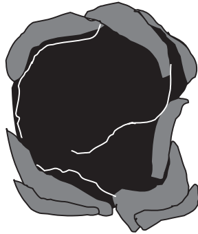
Fig. 15-3. Spheroidal weathering flakes away curved layers of rock.
