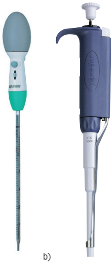
Fig. 133 Pipettes a) measurement pipette made of glass with rubber suction bulb; b) manual pipette with replaceable tip
