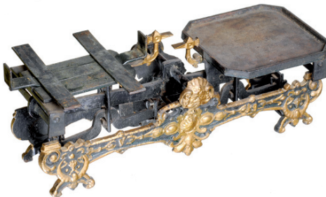
Fig. 19c Lever system of a Béranger flat-pan scale
