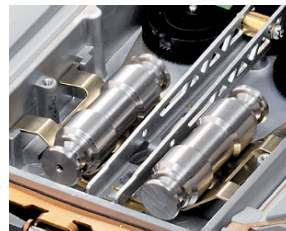
Fig. 139 Reference weights built into the weighing instrument for adjusting the sensitivity
