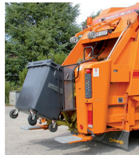
Fig. 75 Garbage truck with integrated scale (Image by courtesy of Digisens AG, Murtlen, CH)
