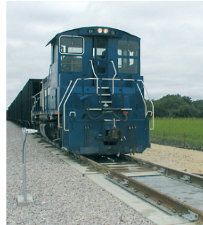
Fig. 12 Rail scale with a weighing capacity of up to 400 t
