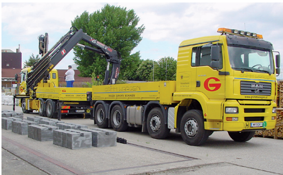
Fig. 156 Standard test vehicle Verification of a bridge scale with standard weights. (Image by courtesy of Grimm Waagen, Tresdorf bei Korneuburg, AT)
