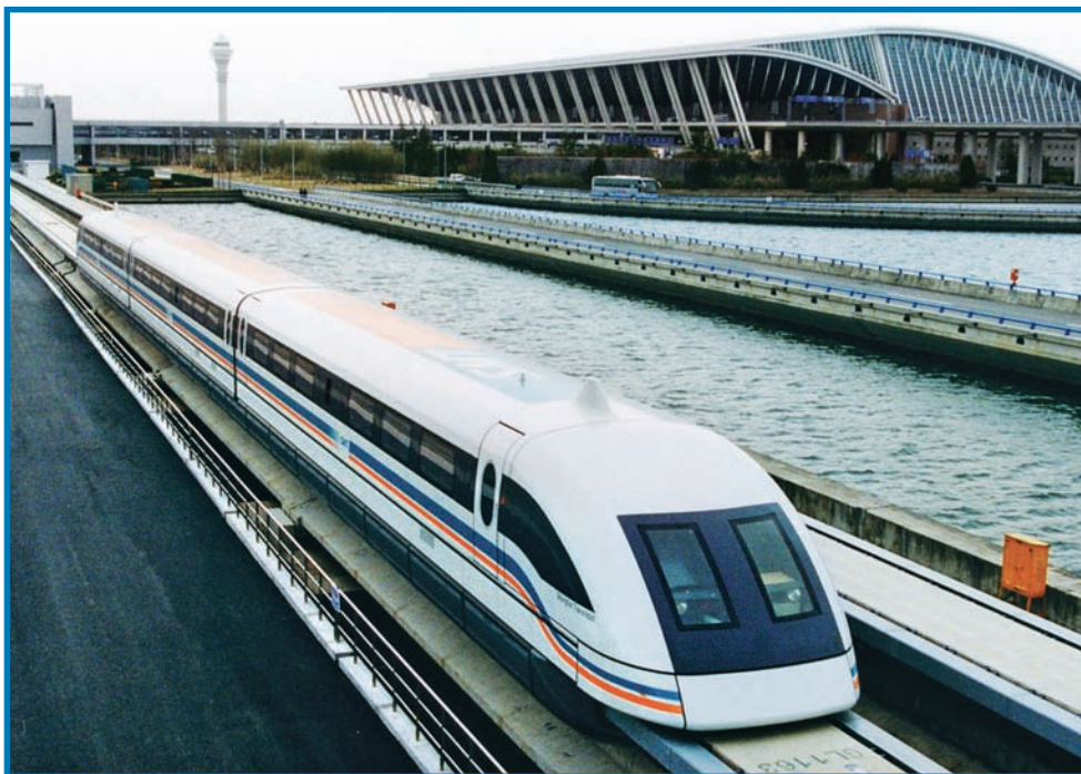
Figure 5.2 Scientists have created a means of revolutionary train travel. The “levitation” train travels over superconducting metal. This metal concentrates electricity so that it becomes an intense magnetic field. Magnetic parts in the train make the train levitate and travel at speeds close to 350 miles per hour.
