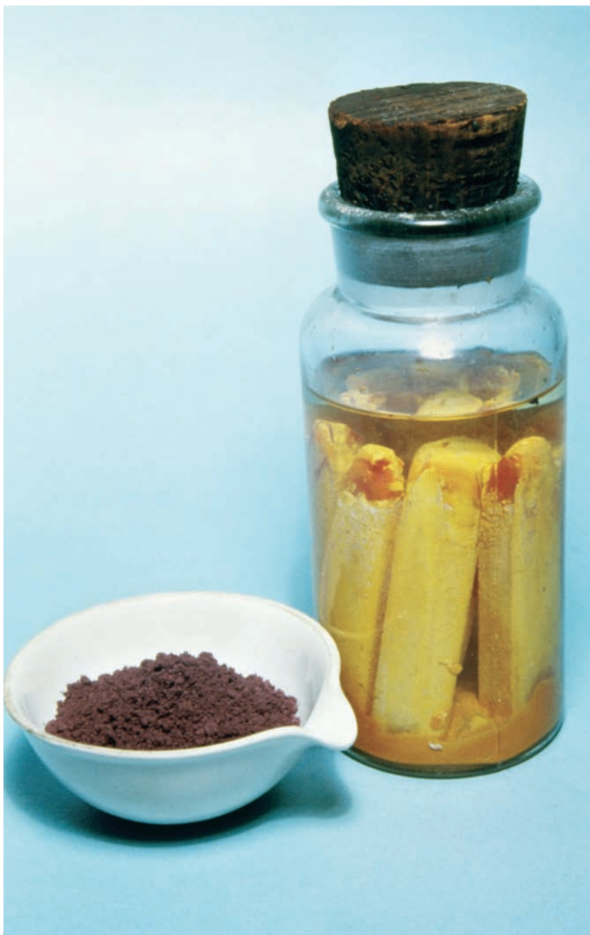
Elemental phosphorus comes in red and white forms. (Richard Treptow/Photo Researchers, Inc.)
