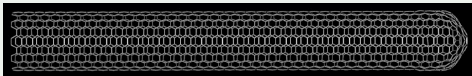
FIGURE 11.7 A portion of a nanotube. The closed end is approximately one half of a buckyball. The main length cannot close as long as all of the rings are hexagons.
