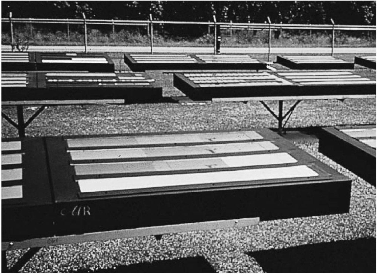
FIGURE 19.8 Paint panels exposed under “black box” conditions. [Picture courtesy of Atlas Weathering Services Group]
