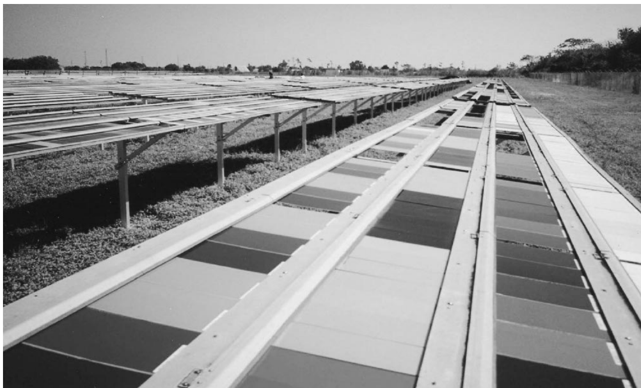
FIGURE 19.5 Paint test panels exposed at 5 degrees facing south. [Picture courtesy of Q-Panel Company]
