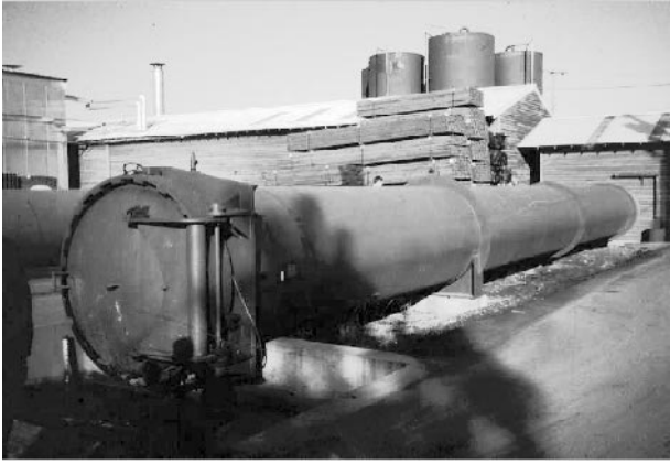
FIGURE 15.9 Example of a pressure treatment cylinder.
