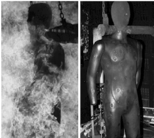
FIGURE 13.12 (a) Pyroman fully engulfed in flames; (b) Bare pyroman.
