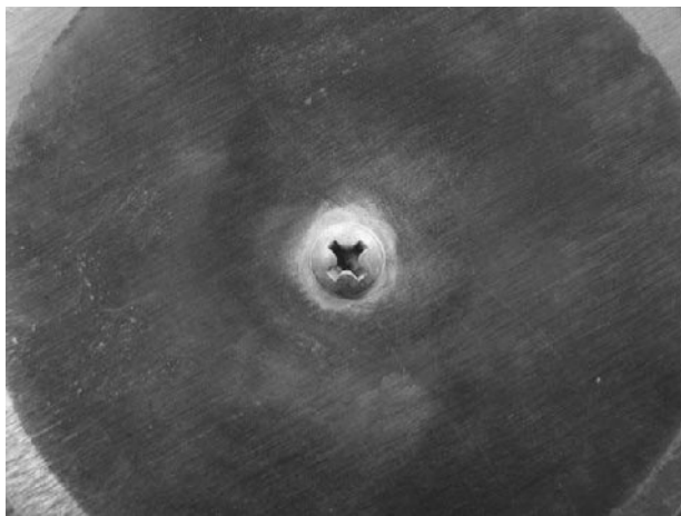
FIGURE 27.12 Galvanic corrosion where a large anode area is in contact with a small cathode area.
