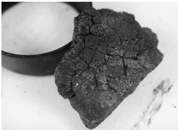
FIGURE 2.17 A sample of a coke lump collected from the inside surface of the radiant coil.
