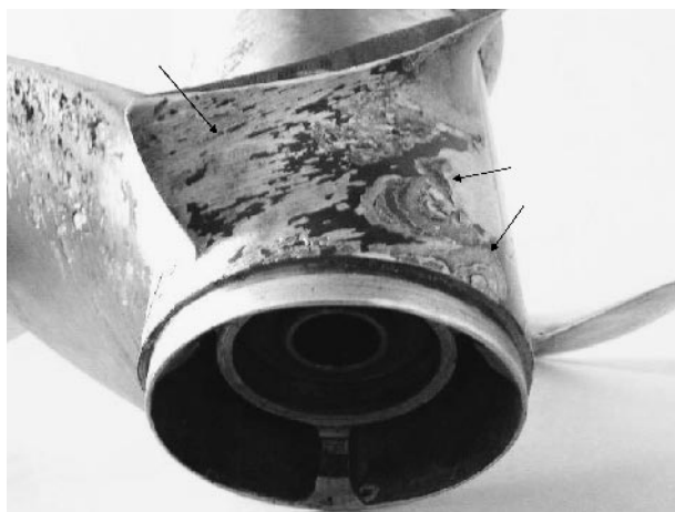
FIGURE 27.5 Cavitation corrosion of a stainless steel propeller.
