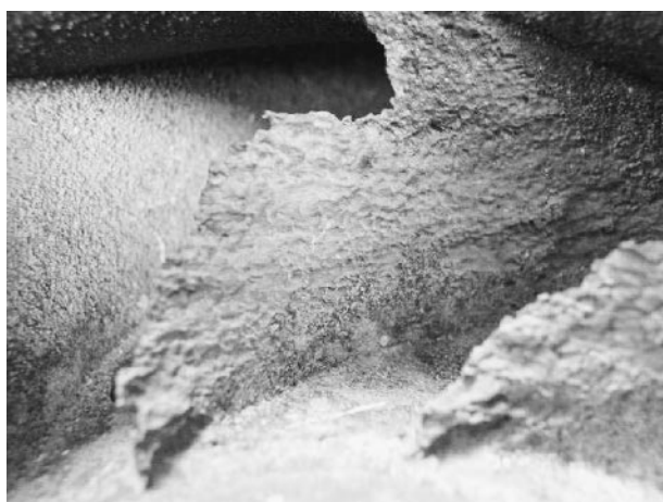
FIGURE 27.6 Erosion corrosion of a brass water pump. (Top) Photograph showing all of the corroded pump impellers. (Bottom) Close-up of the erosion corrosion on one of the pump impellers.
