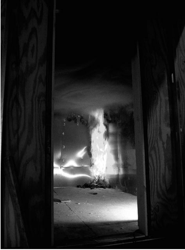
FIGURE 10.6 ISO 9705 room/corner test in progress.
