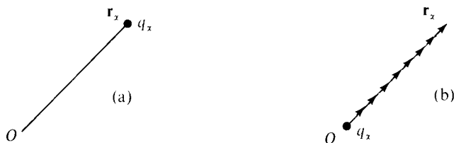
Figure 1. The real charge distribution q_\alpha at \mathbf{r}_\alpha , represented in (a), is equivalent to the reference distribution ( q_\alpha at O ) plus n dipoles q_\alpha \mathbf{r}_\alpha/n (b).
