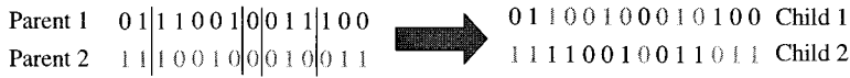
Figure 6.16 In n-point crossover, n points in the vector are randomly chosen, and crossover is performed to produce two new children.
