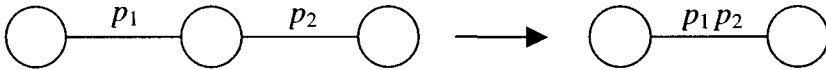
Figure 6.62 This is an illustration of the series reduction that is used in the Factor algorithm.
