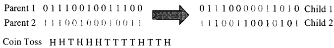
Figure 6.17 In uniform crossover, a coin is flipped for each switch state. For heads, the first child gets the first parent’s switch state, and the second child gets the second parent’s switch state. For tails, the opposite action is taken.
