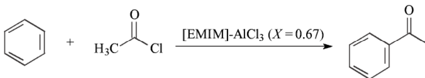
Scheme 5.1-62: The acetylation of benzene in a room-temperature ionic liquid.
