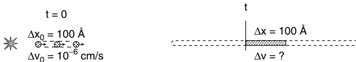
Figure 25. The uncertainty in position for the electrons is \Delta x_0 \sim 100 \text{ \AA} at the time of emission. A certain time t later, a piece of size \delta x_0 \sim 100 \text{ \AA} is chopped from the extended packet.
